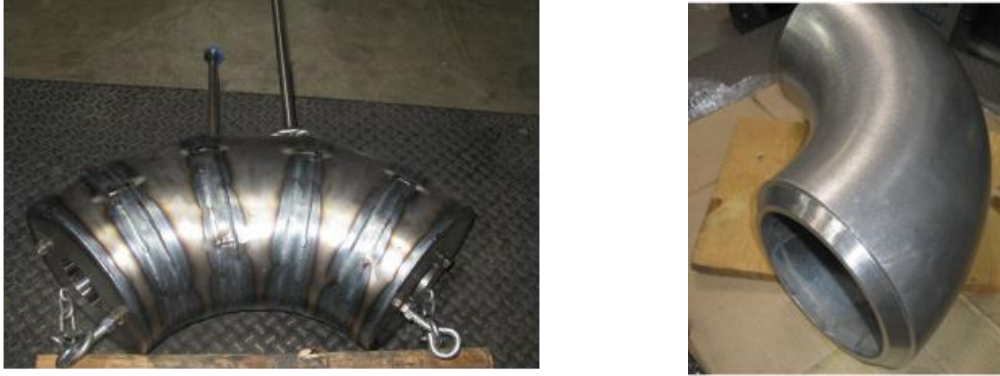
Figure 11. Left: Fabricated and filled can prior to HIP, Right: Machined and heat treated elbow.
