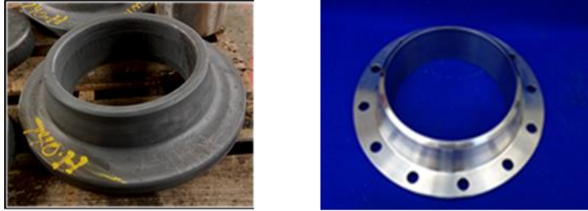
Figure 9. Weld neck flange hammer forged at Maass Flange Corporation, Sealy TX, Left: as forged, Right: Machined flange.
