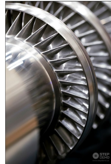
Close up of EDM Turbine Blades with Spline Test Piece
