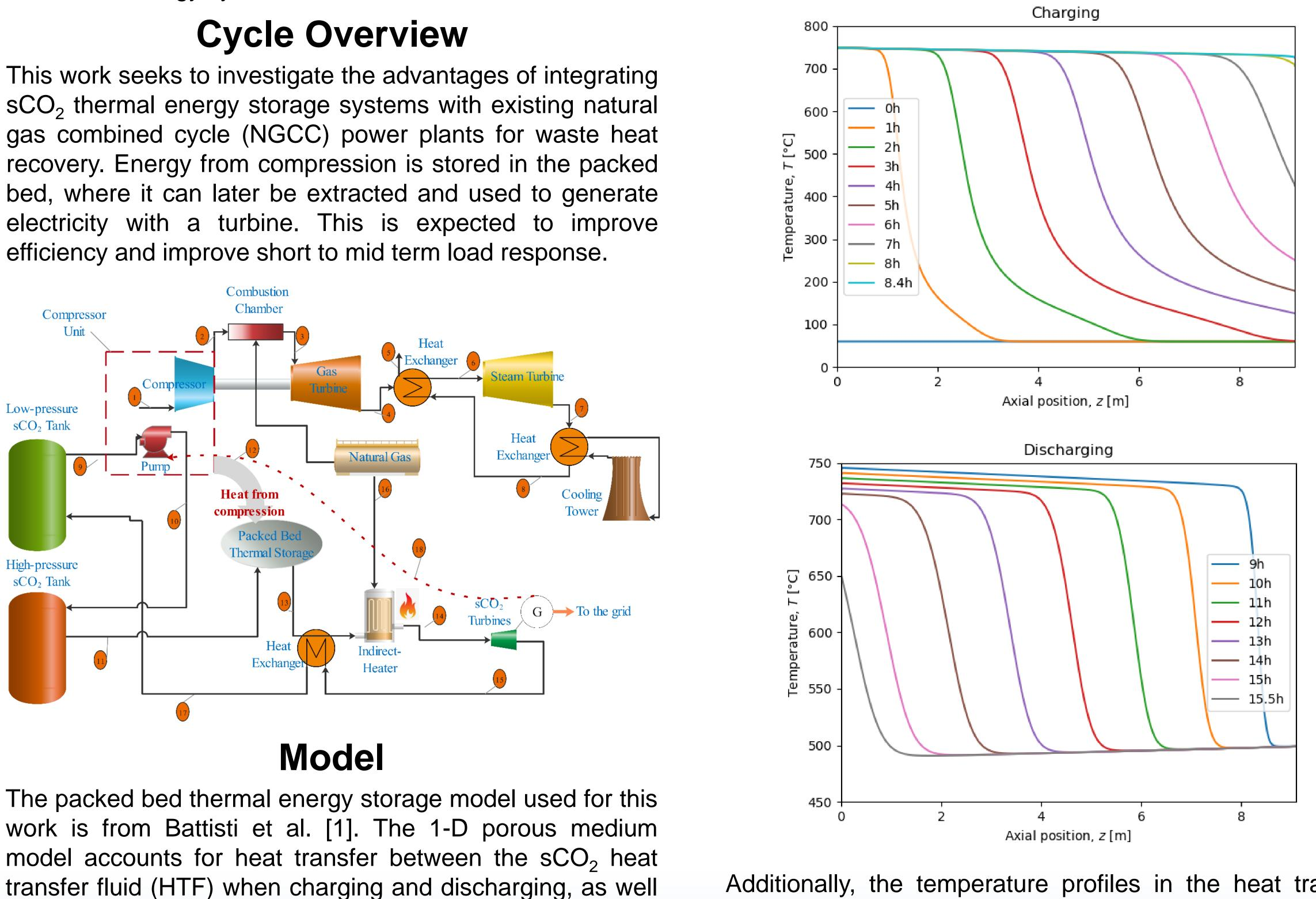
as heat loss to the walls/lids of the tank and its surroundings. This model was implemented in Python for the present work.
