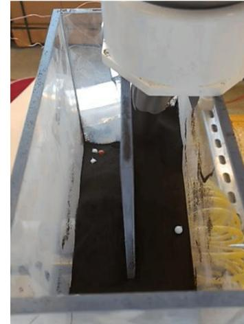
Tests show that a particle gradient forms as the particulate flows through the system.
