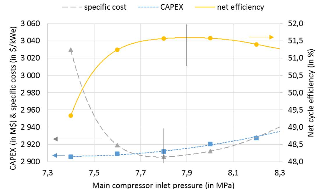
Figure 2: Net cycle efficiency [1] as a function of the main compressor inlet pressure (yellow solid line, right axis), CAPEX (blue dotted line, left axis) and specific costs (gray dashed line, left axis)
