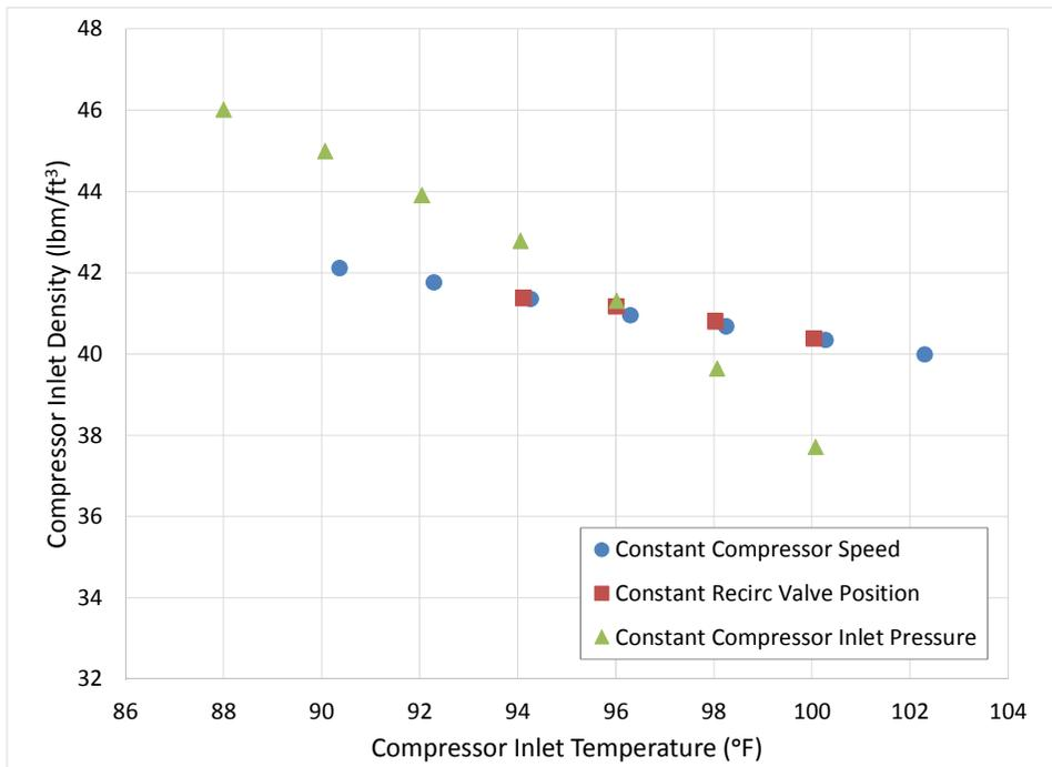
**Fig. 3 Compressor Inlet Density Sensitivity to Compressor Inlet Temperature**
