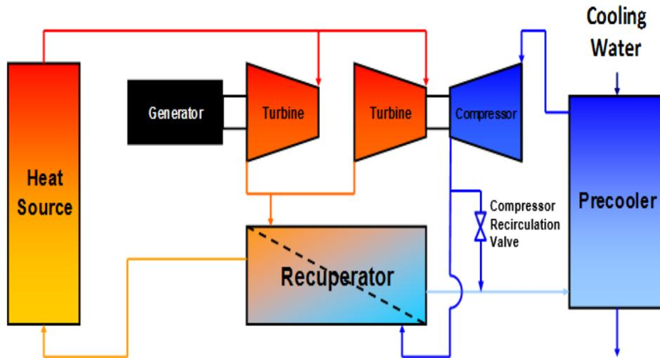
**Fig. 1 IST simple recuperated Brayton Cycle**
