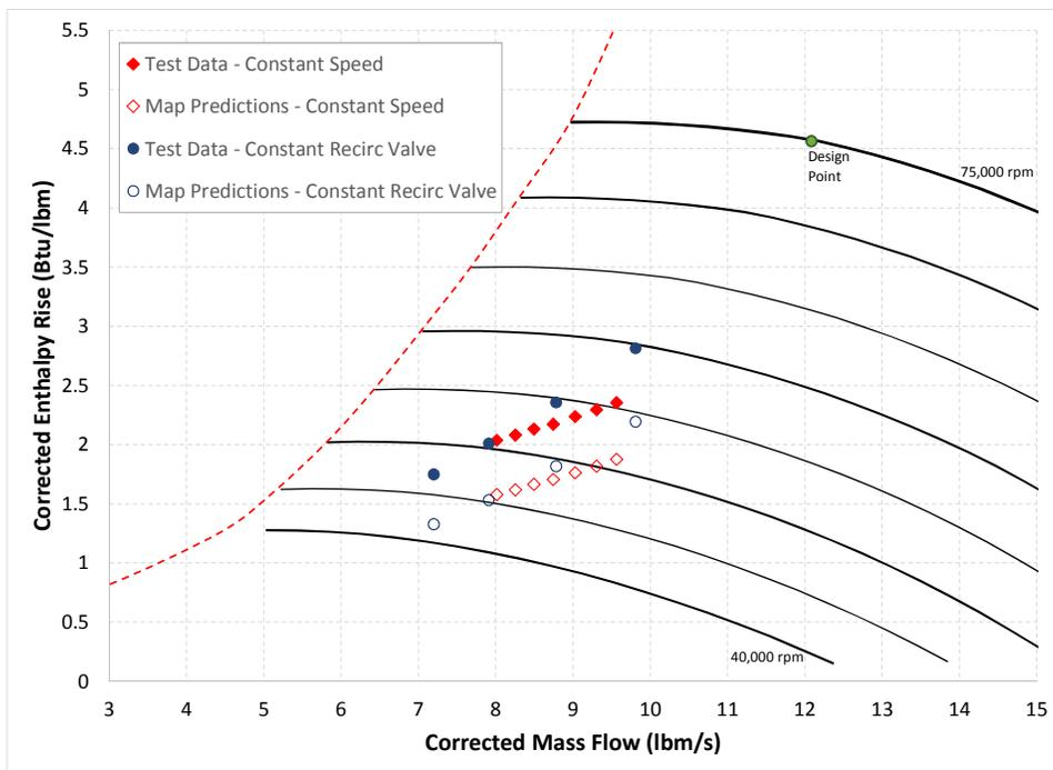
**Fig. 8 Comparison of Compressor Performance to Map Predictions**
