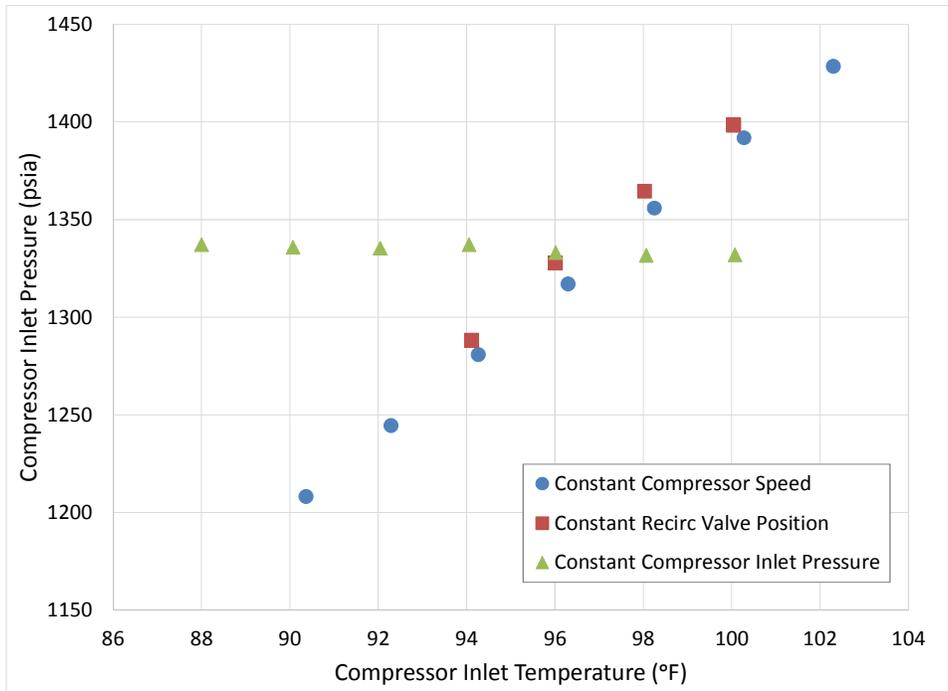
**Fig. 2 Compressor Inlet Pressure Sensitivity to Compressor Inlet Temperature**
