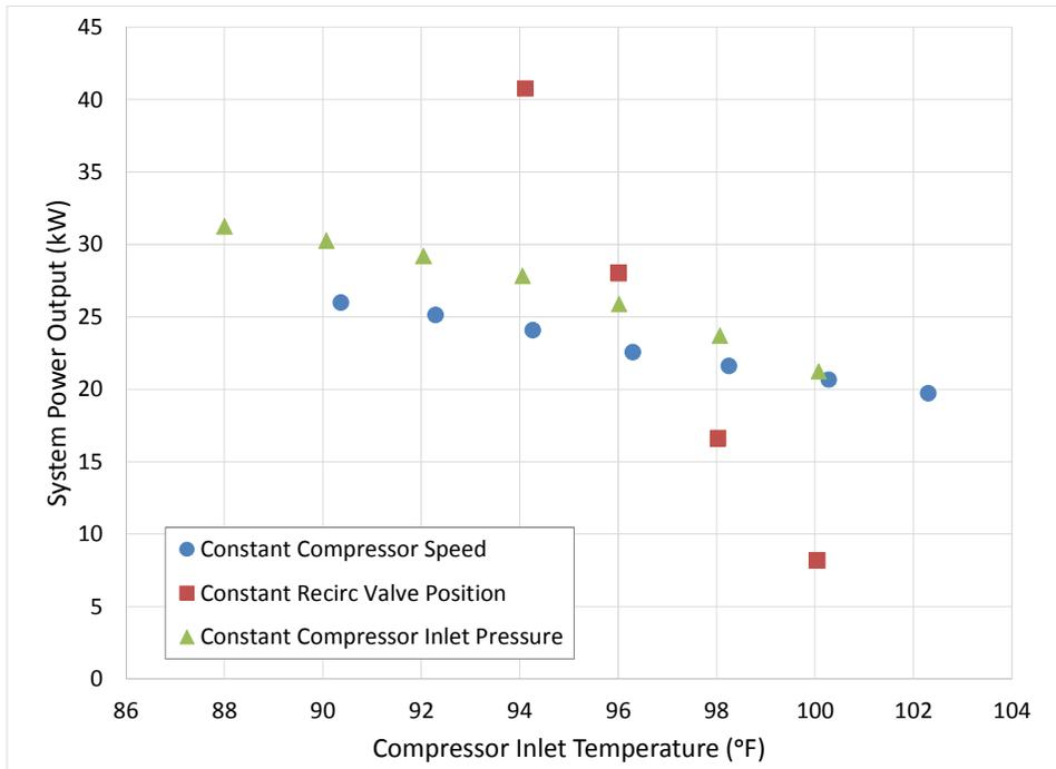
**Fig. 4 System Power Output Sensitivity to Compressor Inlet Temperature**
