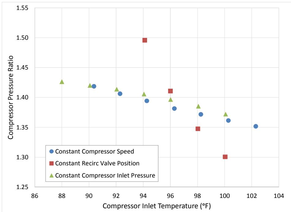
**Fig. 7 Compressor Pressure Ratio Sensitivity to Compressor Inlet Temperature**
