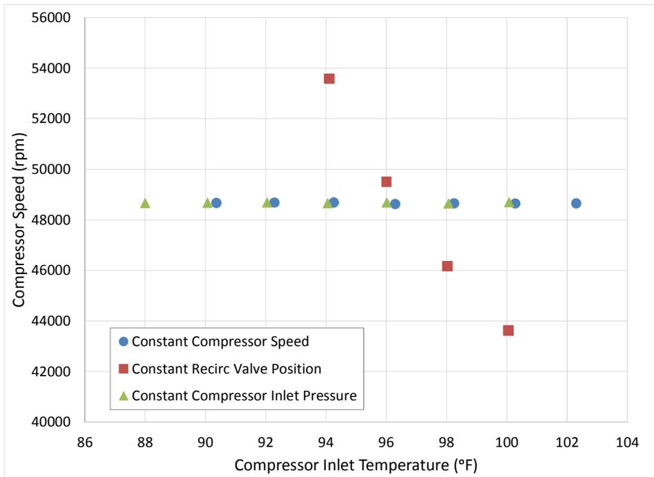
**Fig. 6 Compressor Speed Sensitivity to Compressor Inlet Temperature**
