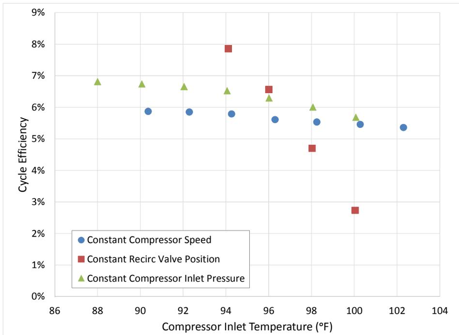
**Fig. 5 Cycle Efficiency Sensitivity to Compressor Inlet Temperature**
