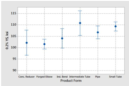
Figure 20. Room temperature 0.2% offset yield strength of heat-treated fittings. ASME min. 90 ksi.
