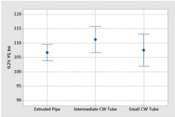
Figure 4. Room temperature 0.2% offset yield strength range of tube and pipe. ASME min. 90 ksi.
