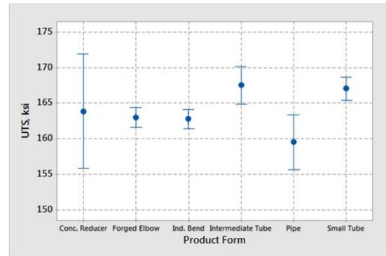
Figure 21. Room temperature tensile strength of heat-treated fittings. ASME min. 150 ksi.
