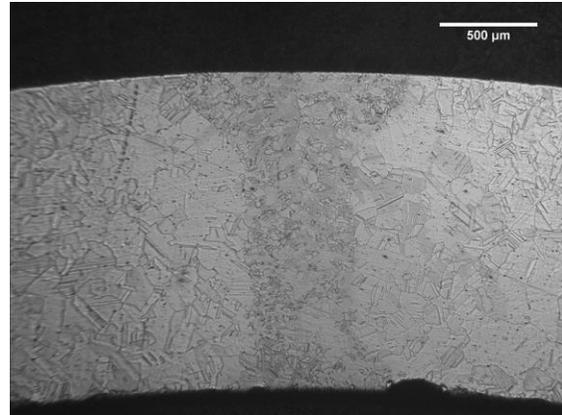
Figure 13. Weld microstructure, off-line continuous anneal
