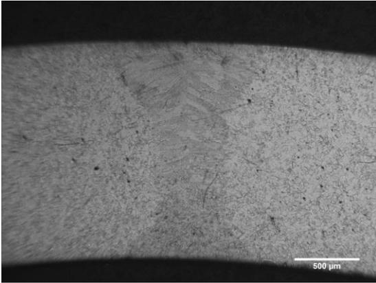
Figure 12. Weld microstructure, In-line continuous anneal.
