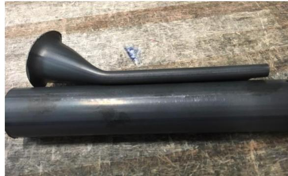
Figure 11. Flare/Flattening Test, after 2075°F (1135°C) off-line anneal.
