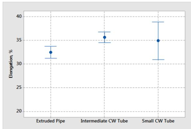
Figure 6 Tensile elongation range of tube and pipe. ASME min. 20%
