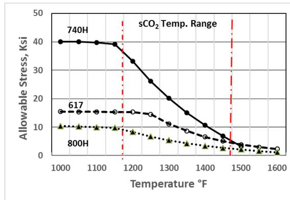
Figure 1. ASME allowable design stress for welded tube and pipe for alloys 740H, 617 and 800HT.
