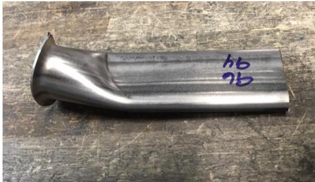
Figure 10. Flare/Flattening Test, welded with flash 1950°F (1066°C) on-line anneal.
