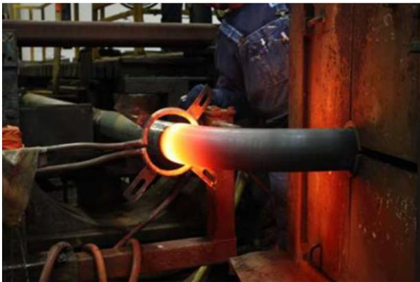
Figure 14. Induction bending at CB&I APP, Clearfield, UT.
