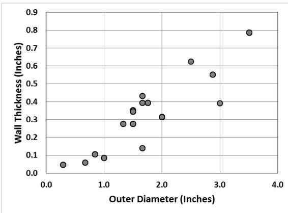
Figure 2. Range of tube OD and wall produced (drawn or pilgered).
