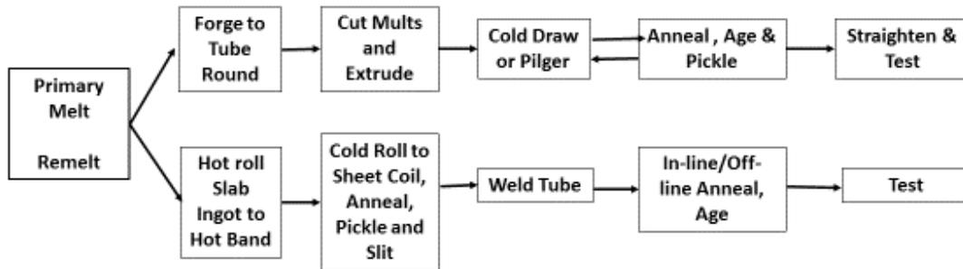
Figure 7. Comparison of seamless and welded tube processes.
