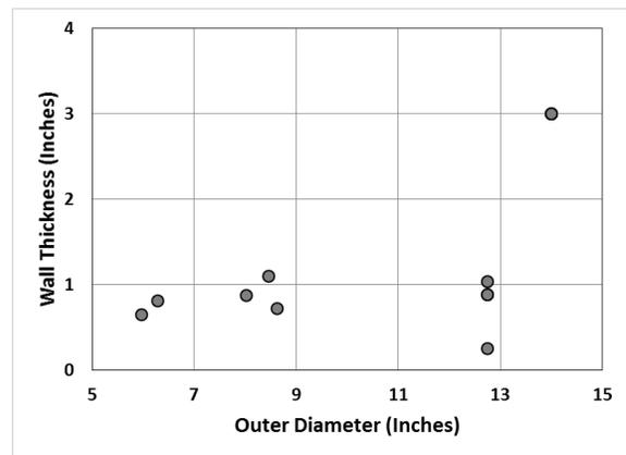
Figure 3 Range of pipe OD and wall produced (extruded or roll formed).
