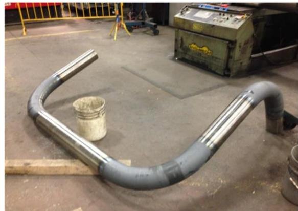
Figure 15 Pipe bends assembled with butt welds.
