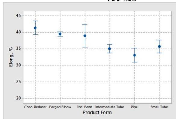
Figure 22. Room temperature tensile elongation of heat-treated fittings. ASME min. 20%.
