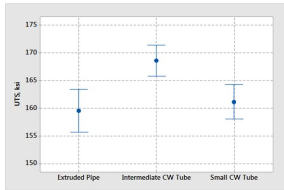
Figure 5. Tensile strength range of tube and pipe. ASME min. 150 ksi.
