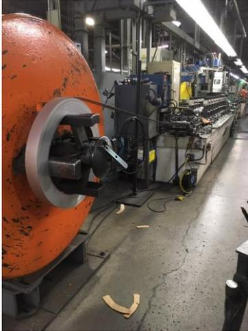
Figure 8. Entry end of tube welding line
