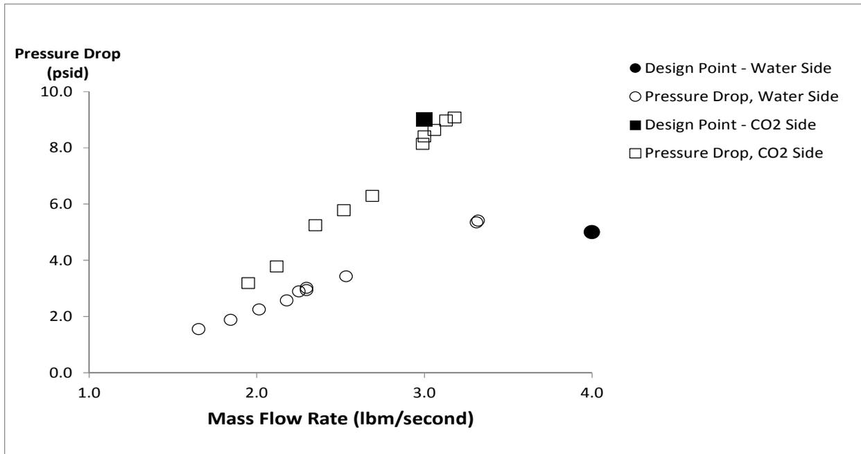
Figure 2. Measured hydraulic resistance of the heat exchanger (expanded uncertainty of the pressure drop is  $\pm 0.003$  psid)
