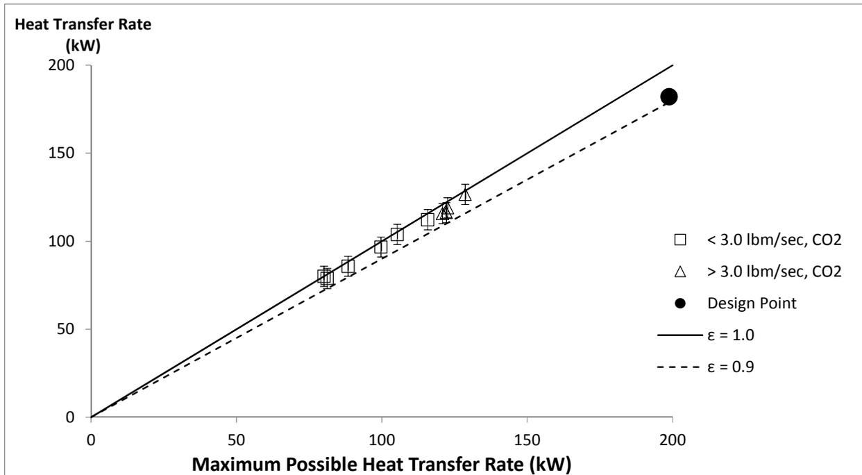
Figure 1. Measured thermal performance showing the effectiveness of the water-to-sCO<sub>2</sub> heat exchanger (expanded uncertainty of the heat transfer rate shown is  $\pm 5.72$  kW - the average of the uncertainties for the CO<sub>2</sub> side and the water side)
