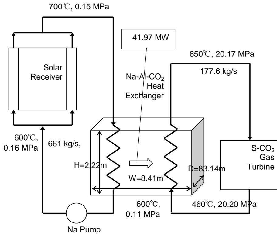
**Fig. 2. Solar thermal power generation system with a Na-cooled receiver, Al heat exchanger, and CO<sub>2</sub> gas turbine.**
