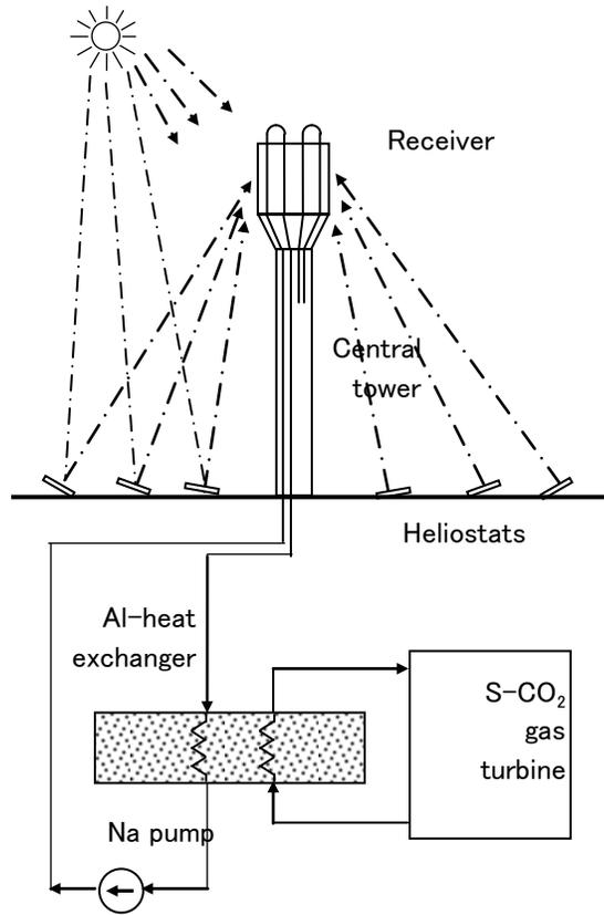
**Fig. 1. Solar thermal power generation system with Na-cooled receiver, Al heat exchanger and CO<sub>2</sub> gas turbine.**
