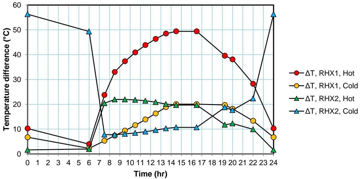
Fig. 7. Histories of end temperature differences of the recuperators for partial load operation.
