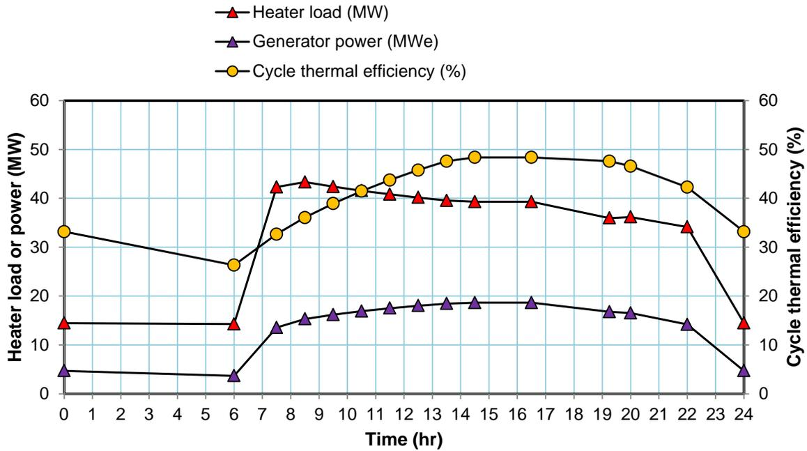
Fig. 6. Time histories of the heater load, the generator power and the cycle thermal efficiency for the partial load operation.
