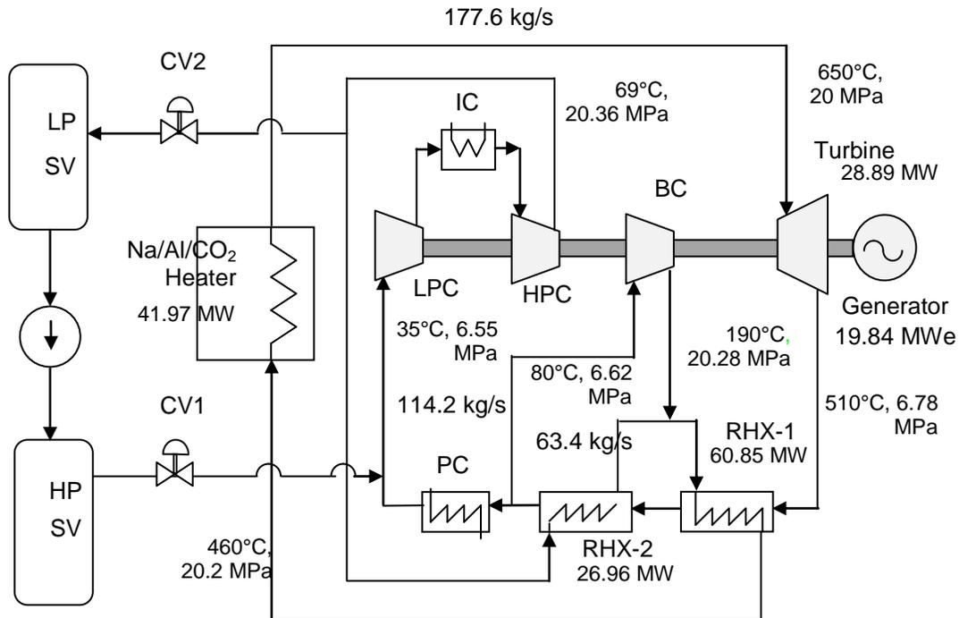
**Fig. 3. Design data for the supercritical CO<sub>2</sub> gas turbine cycle.**
