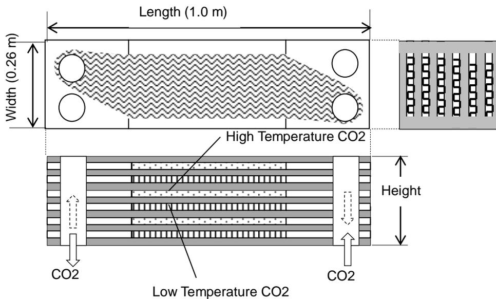
Fig. 4. Structure and dimensions of the PCHE module.
