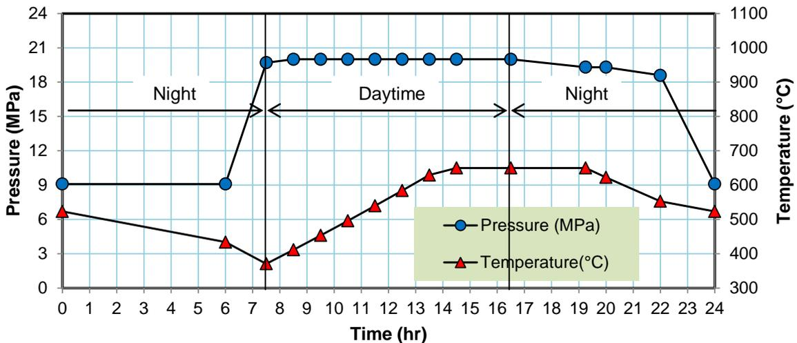
Fig. 5. Time histories of the turbine inlet pressure and the turbine inlet temperature for the partial load operation.
