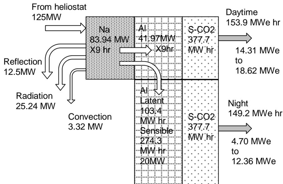
**Fig. 8. Total energy balance of the solar thermal power plant with Na cooled receiver, aluminum heat storage and S-CO2 GT.**
