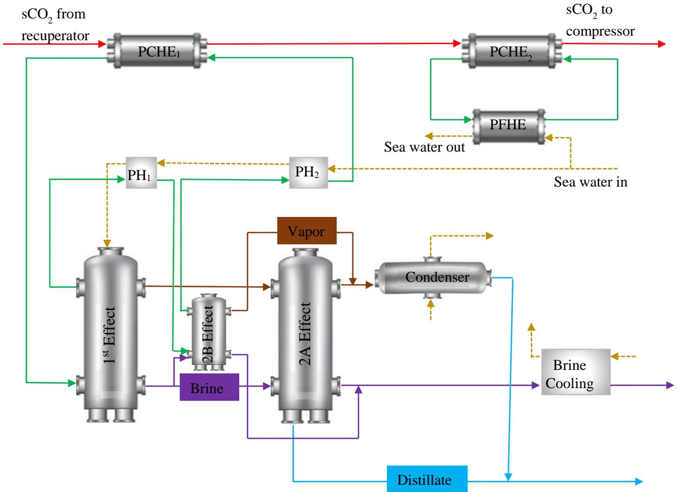
Figure 4: Integration of MED with sCO<sub>2</sub> Brayton cycle via intermediate sensible heating evaporators.
