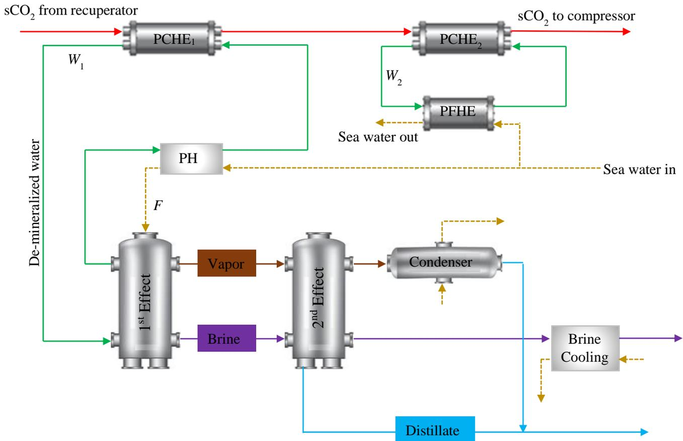
Figure 1: Schematic for forward feed MED integrated with  $s\text{CO}_2$  recompression cycle.
