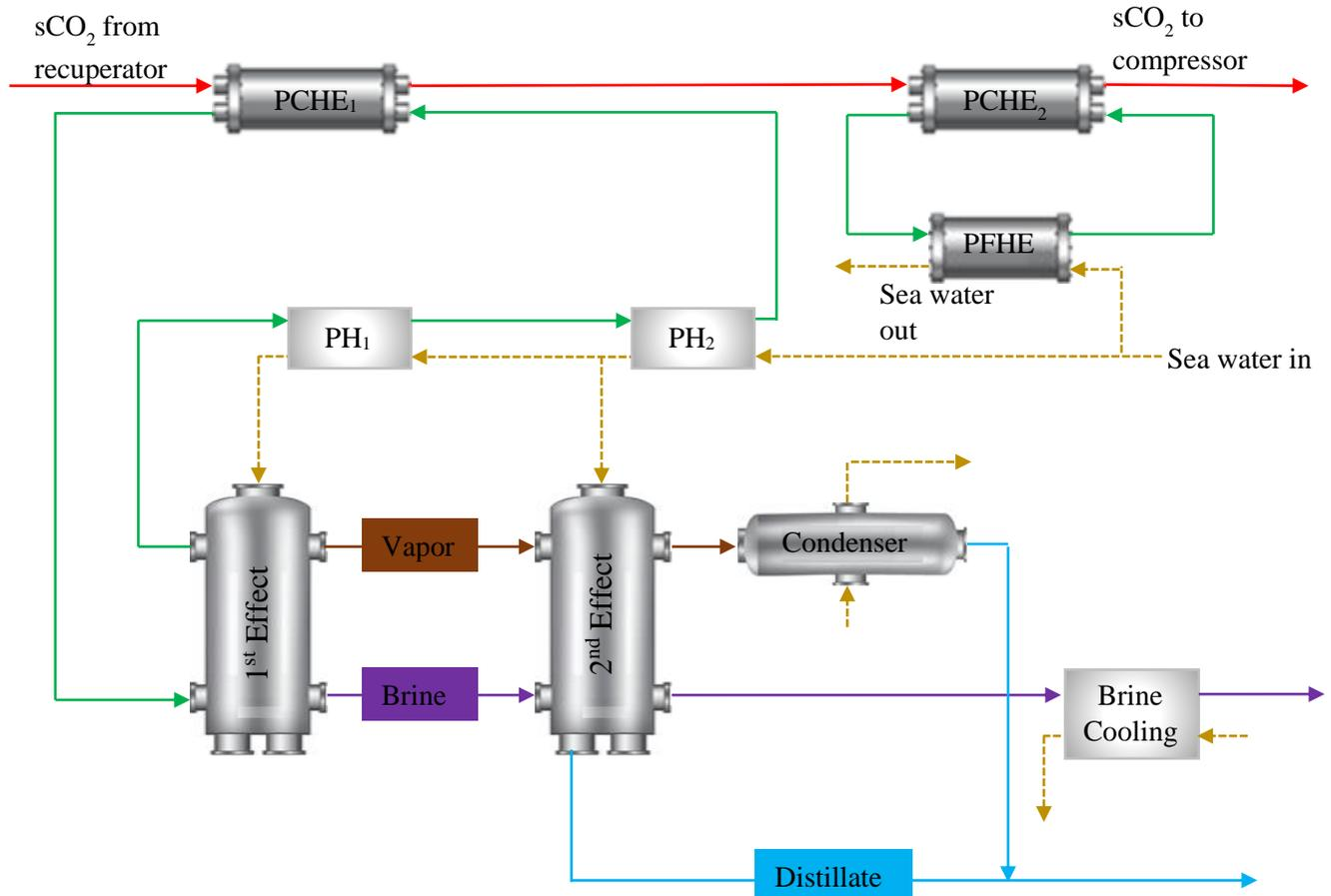
Figure 2: Schematic for parallel/cross feed MED integrated with  $s\text{CO}_2$  cycle.
