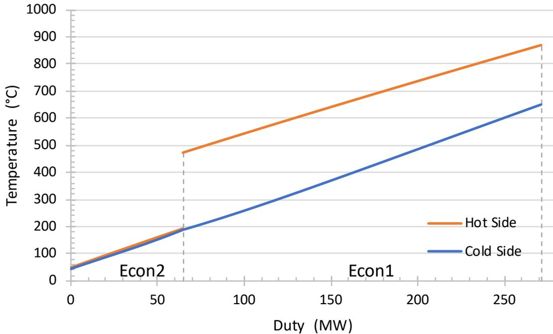
Composite curves are much closer than in the Baseline Case indicating a lower average driving force for heat transfer but a higher recuperator effectiveness. However, for the economizers, this situation is reversed which acts to negate the benefit of a higher recuperator effectiveness.
