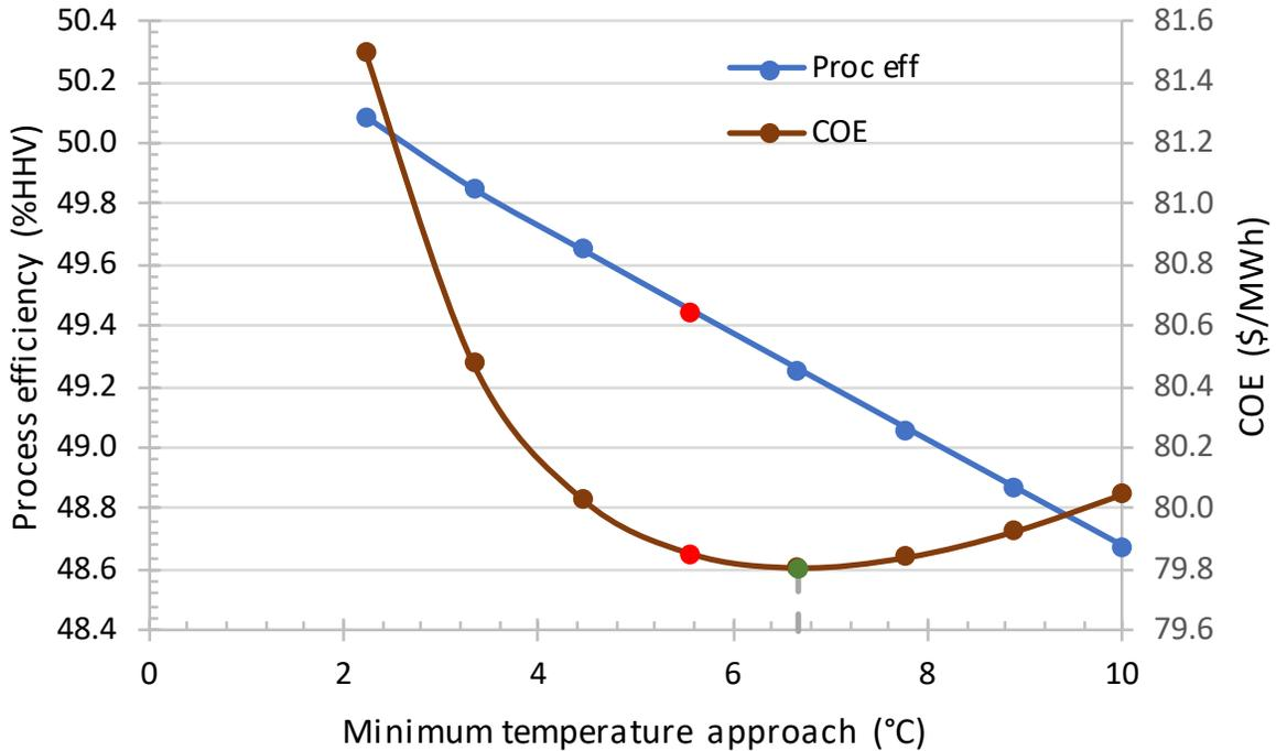
The results show that the process efficiency decreases monotonically and almost linearly with increasing minimum temperature approach whereas the COE passes through a minimum at a temperature approach of 6.7 °C (gray dashed vertical line and green marker). While this result suggests that a lower COE could be attained with a higher minimum temperature approach of 6.7 °C, the 0.2 percentage point drop in process efficiency was deemed more significant than the negligible drop in COE.
