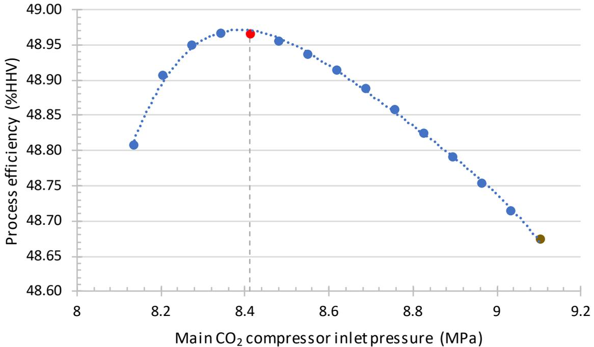
This performance only sensitivity analysis showed that the maximum process efficiency was attained using a compressor inlet pressure of 8.41 MPa. This yielded an optimum cycle pressure ratio of 4.1.
