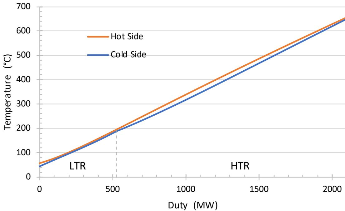
**Figure 10 Economizer T-Q diagram for the Alternate Configuration Case**
