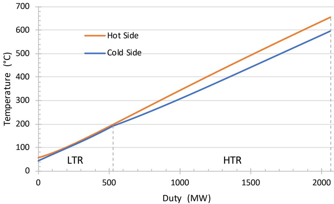
Figure 8 Economizer T-Q diagram for the Baseline Case
