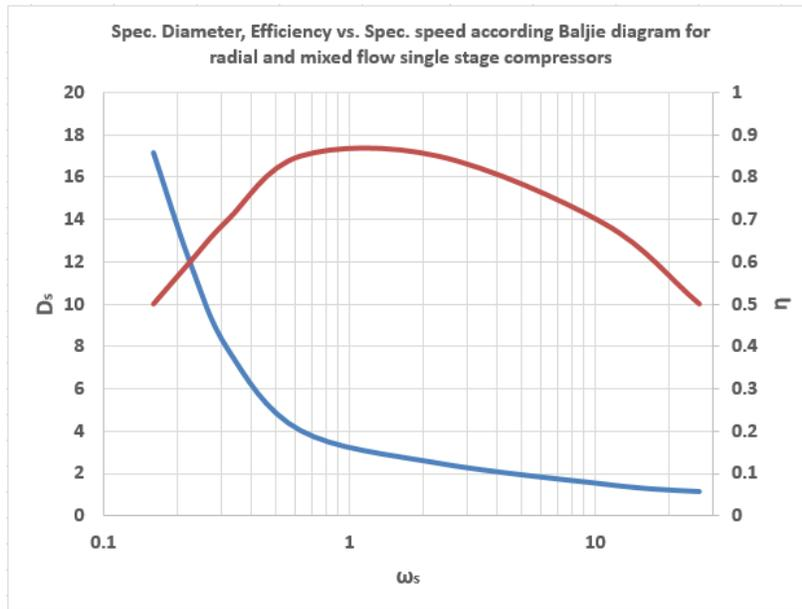
Fig. (6) – Specific diameter vs. specific speed extracted from Balje diagram for radial and mixed flow single stage compressors
