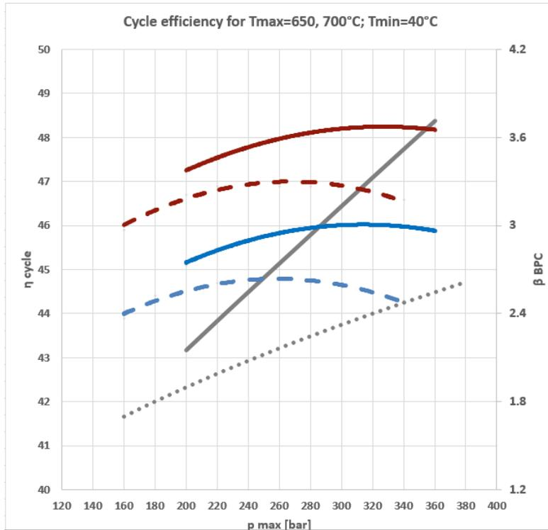
Fig. (3) – Thermal cycle efficiency with 650, 700°C of maximum temperature and corresponding BPC pressure ratio
