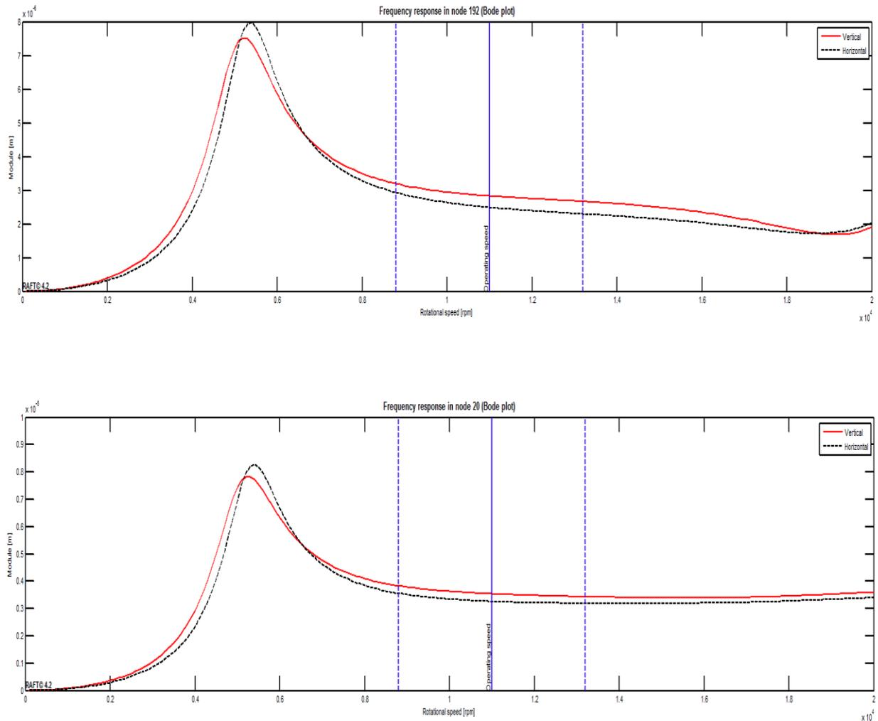
Fig. (4) – Frequency response @: exhaust side guide bearing (upper), inlet side guide bearing (lower)
