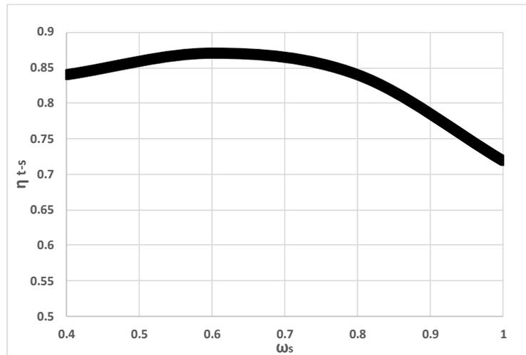
Fig. (7) – Typical total to static efficiency vs. specific speed for radial single stage turbines
