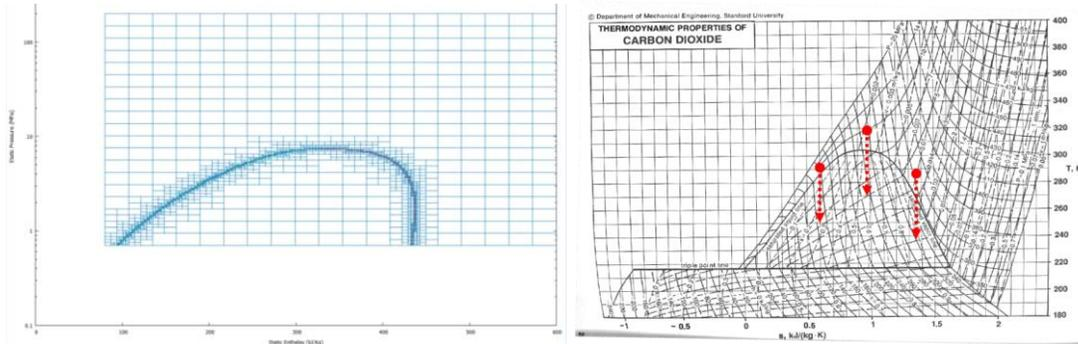
**Plot of selectively refined thermodynamic table now used in Concepts NREC software (left) and paths of 1D nozzle flows over the thermodynamic map**
