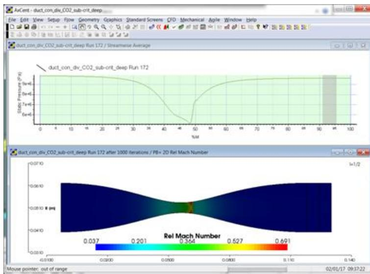
**CFD results of a sCO<sub>2</sub> nozzle expansion from the liquid side showing atypical results**
