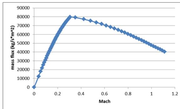
Mass flux as function of Mach number for isentropic expansion through the liquid side of the saturation line
