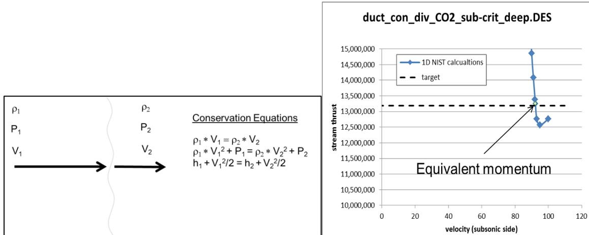
Conservation equations (left) and stream thrust distribution as a function of exit velocity (right)
