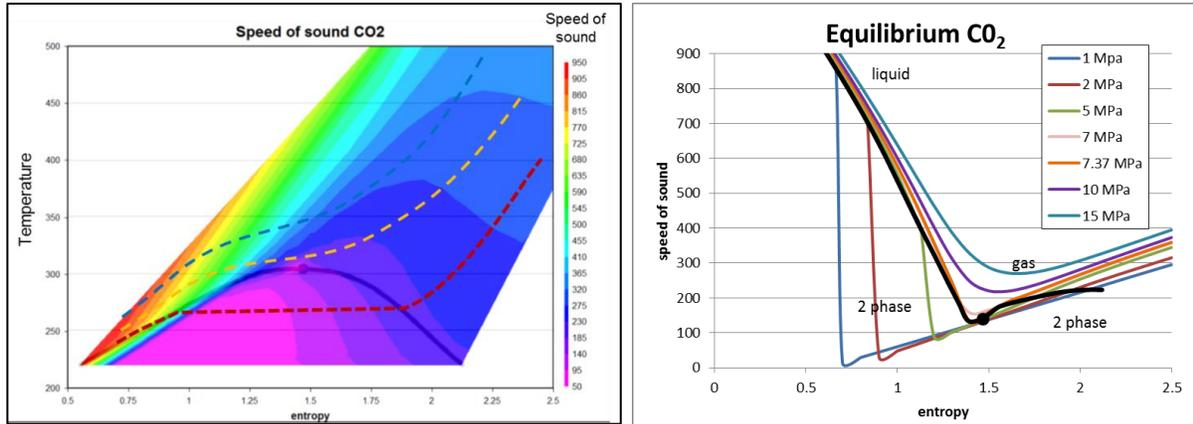
Speed of sound values derived from REFPROP and Brennen
