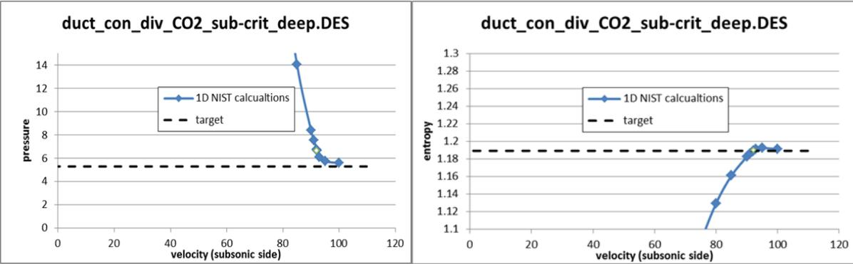
**Iterations in 1D model on velocity to match mass, momentum, and energy across the shockCFD- results of a sCO<sub>2</sub> nozzle expansion from the liquid side showing atypical results**
