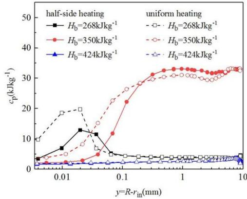
Fig. 3. Specific heat distribution under half-side heating and uniform heating conditions
