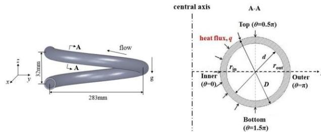
Fig. 1. Physical model of the helical tube
