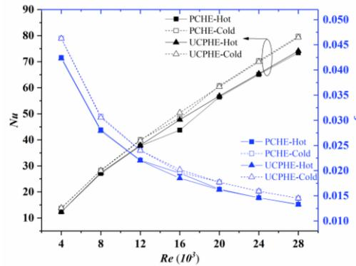
Fig. 7. Comparison between UCPHE and PCHE: Nusselt number and friction factor variation against Reynolds number
