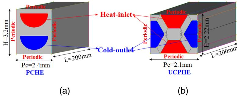
Fig. 6. Numerical model of PCHE (a) and UCPHE (b).
