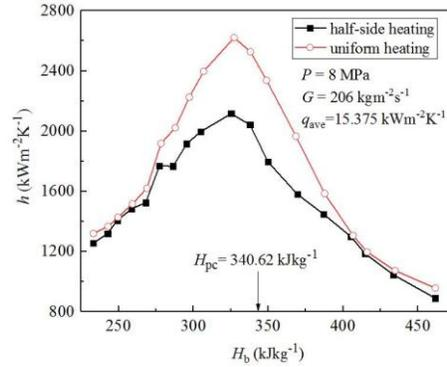
Fig. 2. Heat transfer coefficients under half-side heating and uniform heating conditions
