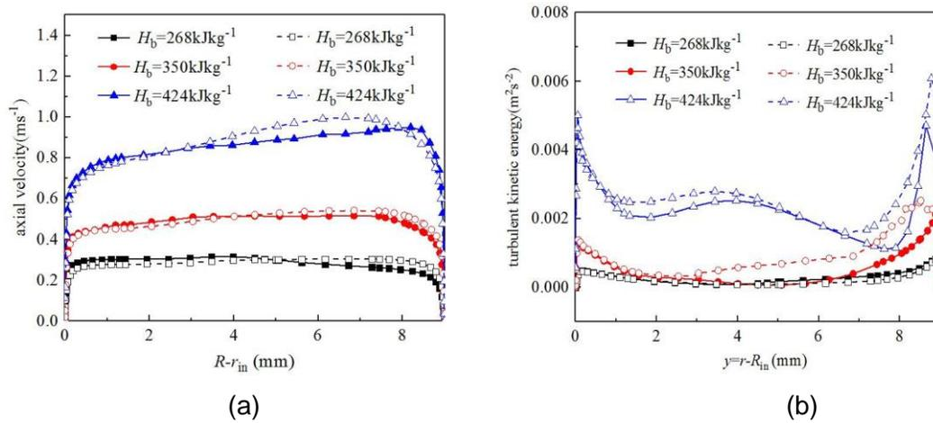
Fig. 4. Streamwise velocity and turbulent kinetic energy distribution under half-side heating and uniform heating conditions.
