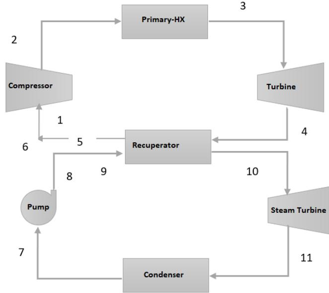
Figure 1: Schematic layout of NTPC Dadri combine plant
