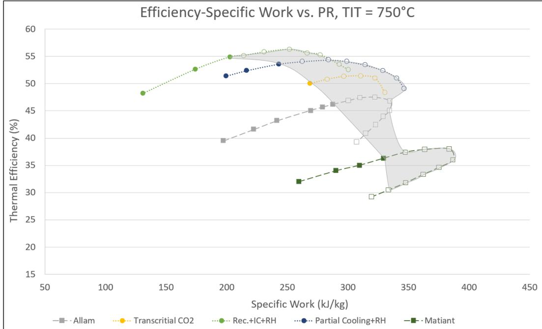
Figure 1: Sánchez et al. studied twelve cycles, five of which promise to yield the greatest gains in thermal efficiency and specific work at 750 °C TIT with forthcoming design and material improvements.
