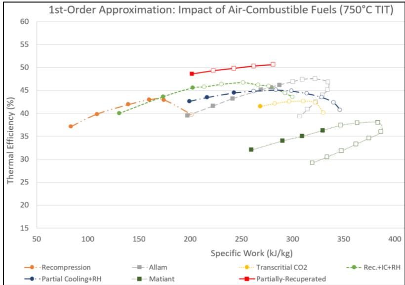
Figure 4: The thermal efficiency of the Partially Recuperated cycle does not suffer when paired with an air-combustible fuel heat source.
