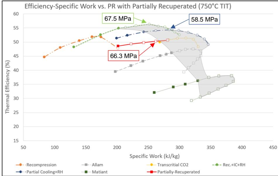
Figure 3: Peregrine’s Partially Recuperated cycle (solid red line, square markers) reaches beyond the Efficiency-Specific Work boundary for 750 °C TIT. Standard Recompression cycle (orange dashed + double dotted line, circular markers) added to contrast with Recompression with Intercooling and Reheat.
