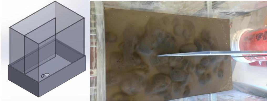
**Figure 5: 1) Cad Design for Single Bend 2) Fluidization of Single Bend**
