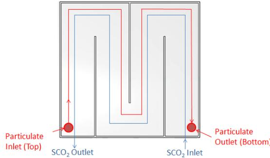
**Figure 1: Axial Counter Flow Fluidized Bed**
