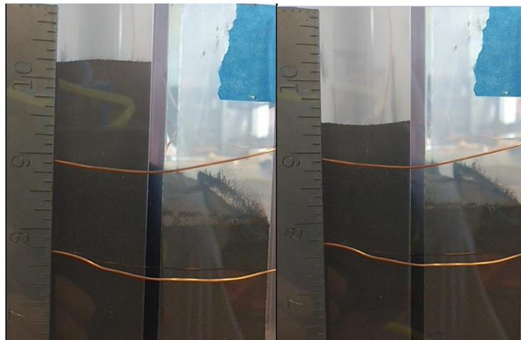
**Figure 4: Steady State Flow Gradient (Side View) a) Low Fluidization b) High Fluidization**
