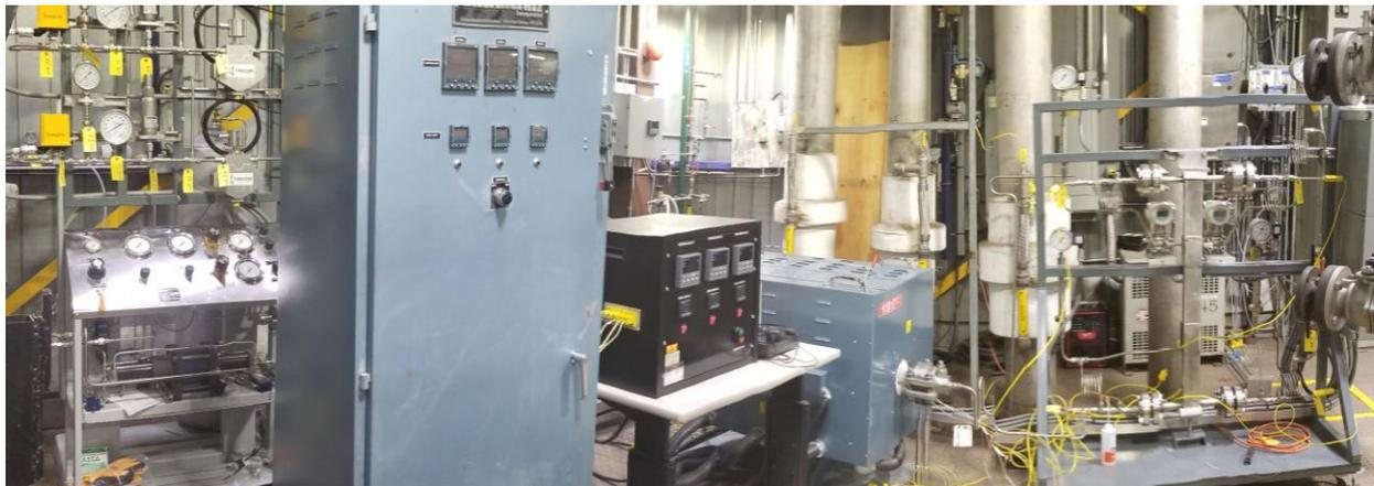
**Figure 2:** CE-O's sCO<sub>2</sub> compact heat exchanger test rig.
