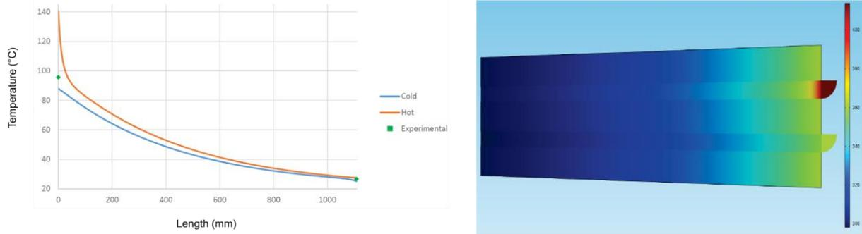
**Figure 3:** Subcritical test results for the PCHE under study.
