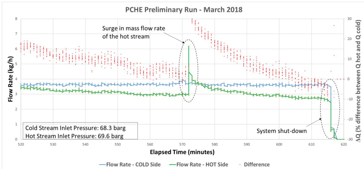
**Figure 5:** Mass flow rate plots and transient response at near critical point.
