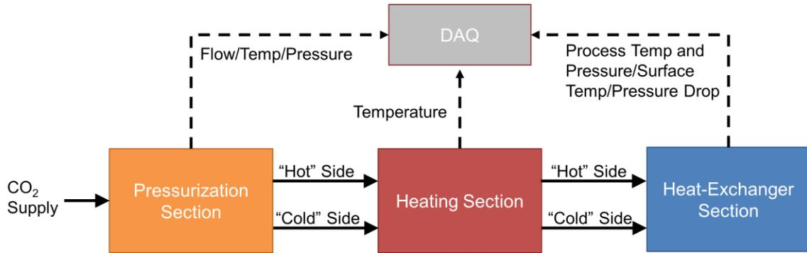
**Figure 1:** Schematic diagram of the process flow for the compact heat exchanger test rig.
