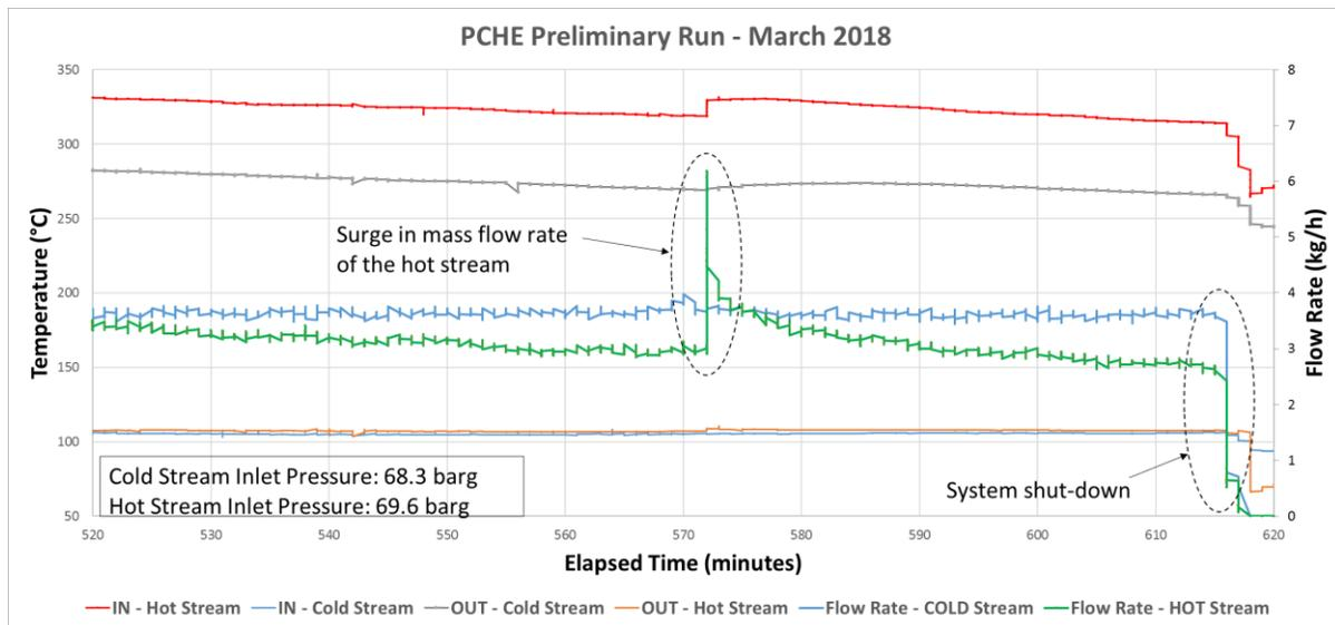
**Figure 4:** Temperature and mass flow rate plots at near critical point.
