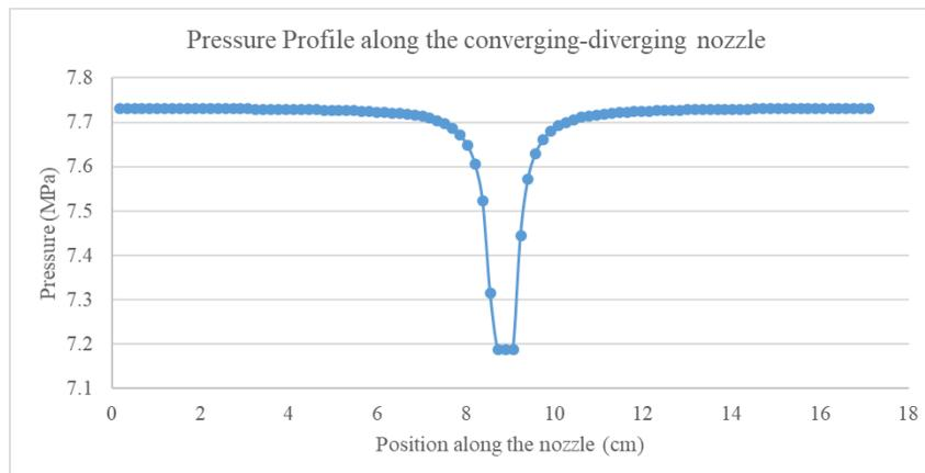
Figure 3b: Pressure Profile along the converging-diverging nozzle
