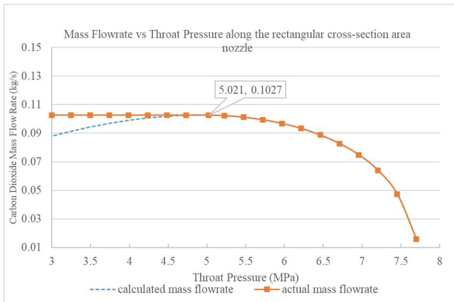
Figure 2: Mass flowrate versus throat pressure in a converging-diverging nozzle; Inlet pressure is 7.4 MPa and temperature is 34.07°C.
