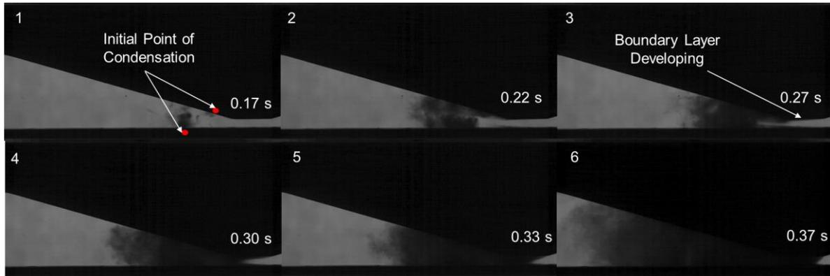
Figure 6: Condensation process captured through high speed camera at 40,000fps
