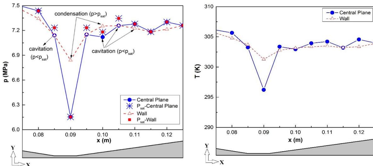
Figure 5: Average pressure (left) and temperature (right) in simulation of condensation behavior at t=2ms
