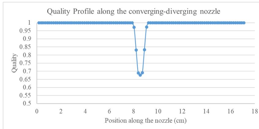
Figure 3c: Quality Profile along the converging-diverging nozzle
