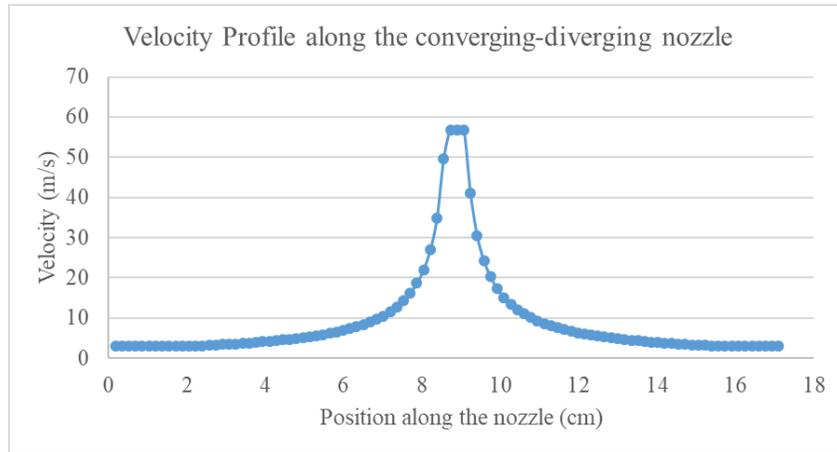
Figure 3a: Velocity Profile along the converging-diverging nozzle
