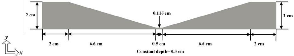
Figure 1: Dimensions of the converging-diverging nozzle used for numerical investigation
