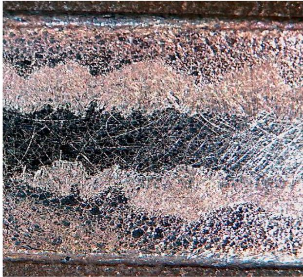
**Figure 3 – Braze Flow from Joints on Vertical-Oriented Face of Insert**
