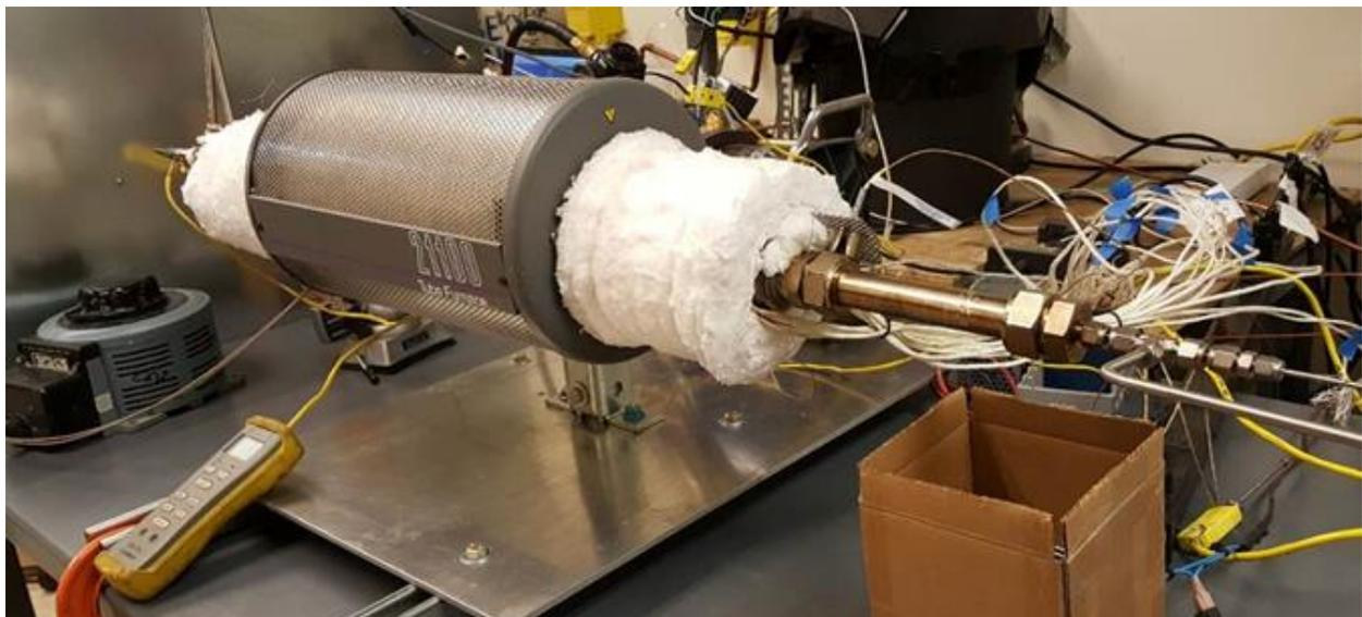
**Figure 4 – High Pressure and Temperature ScCO<sub>2</sub> Test Apparatus**
