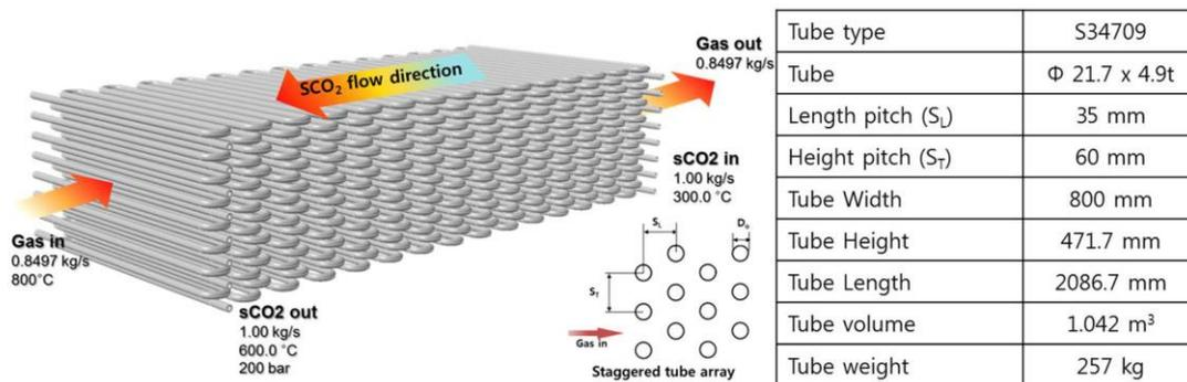
Figure 1. Design of prototype superheater heat exchanger
