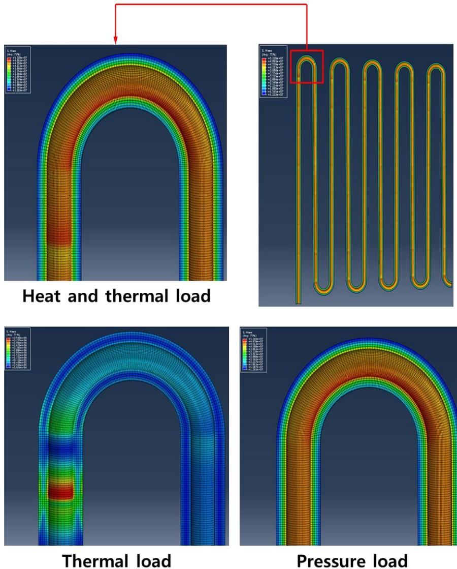
Figure 5. Maximum von-Mises stress location of the tube
