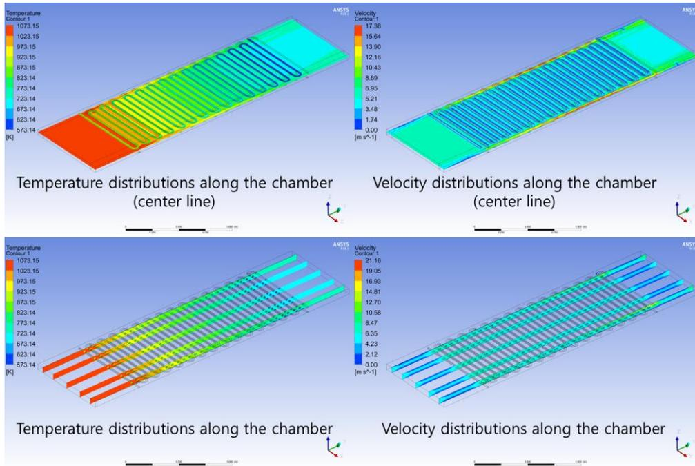
Figure 3. Temperature and velocity distributions along the chamber
