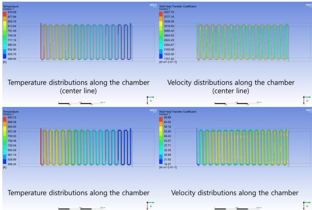
Figure 4. Temperature and velocity distributions along the chamber
