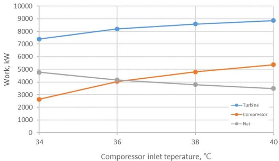
Fig. 3. Turbomachinery work in compressor inlet temperature
