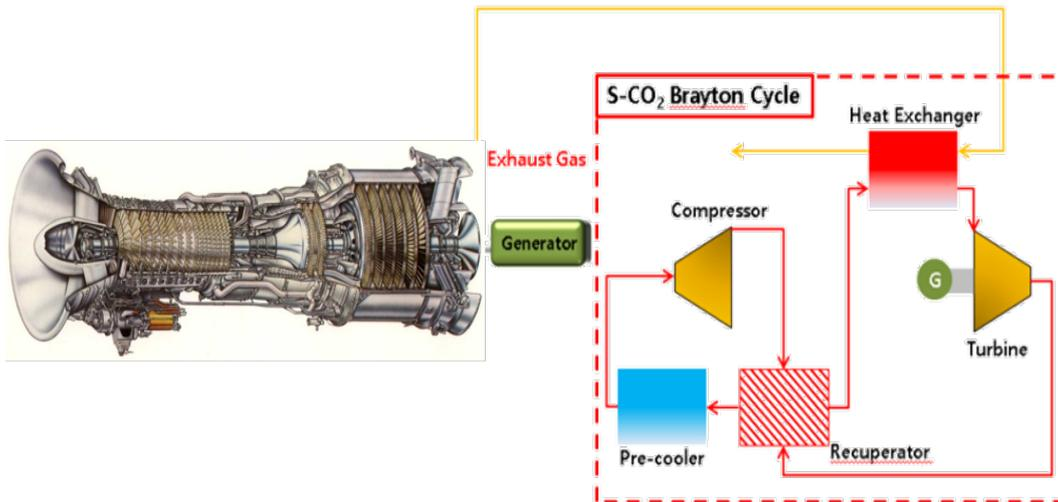
Fig. 1. Supercritical CO<sub>2</sub> cycle layout
