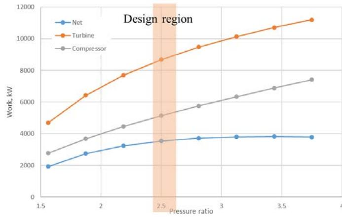
Fig. 2. Turbomachinery work in pressure ratio
