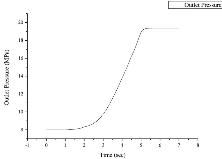
Figure 10. Compressor outlet pressure vs. time during startup
