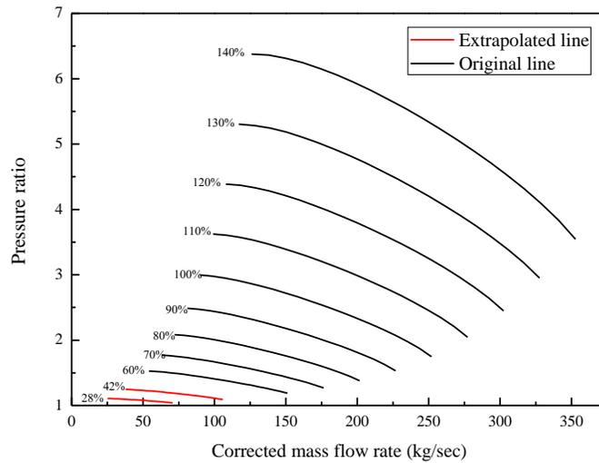
Figure 2. Pressure ratio with respect to corrected mass flow rate of MMR compressor
