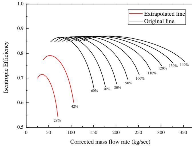
Figure 3. Isentropic efficiency with respect to corrected mass flow rate of MMR compressor
