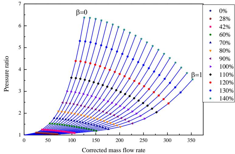
Figure 5. Pressure ratio map with respect to BETA value and compressor rotational speed
