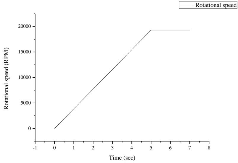
Figure 8. Compressor rotational speed vs. time during startup
