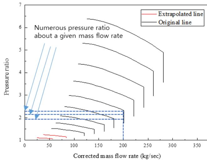
Figure 4. Artificial pressure ratio to show the difficulty of pressure ratio interpolation based on mass flow rate on a steep slope curve
