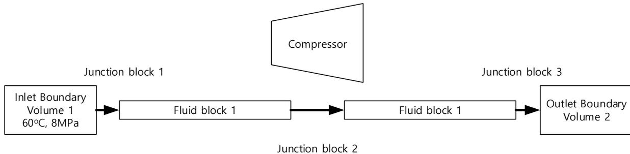
Figure 7. Compressor test section in GAMMA+ code for startup simulation
