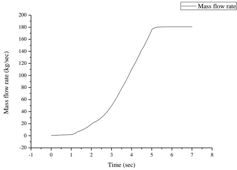
Figure 9. Compressor mass flow rate vs. time during startup
