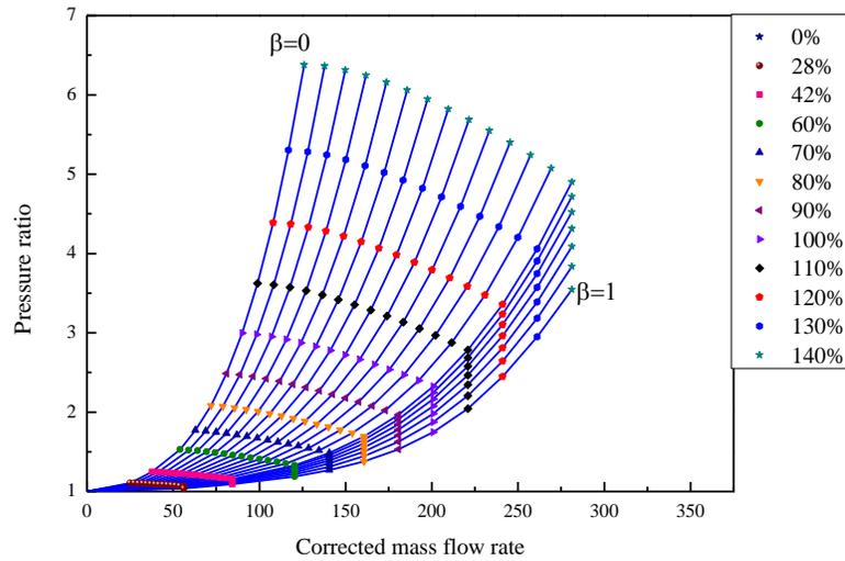
Figure 6. Pressure ratio map with respect to BETA value and compressor rotational speed
