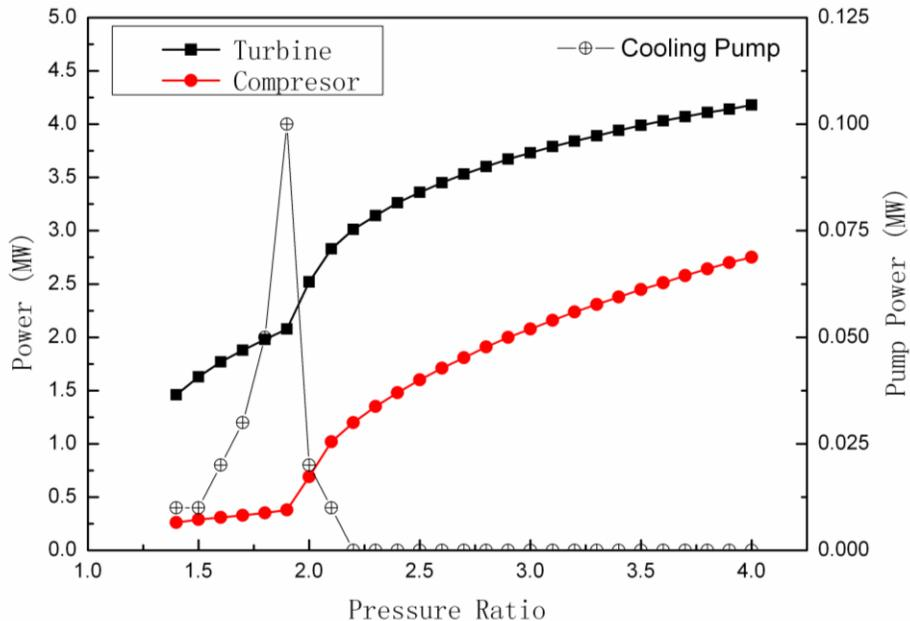
Figure 5 The pressure ratio effect on turbine, compressor and pump power
