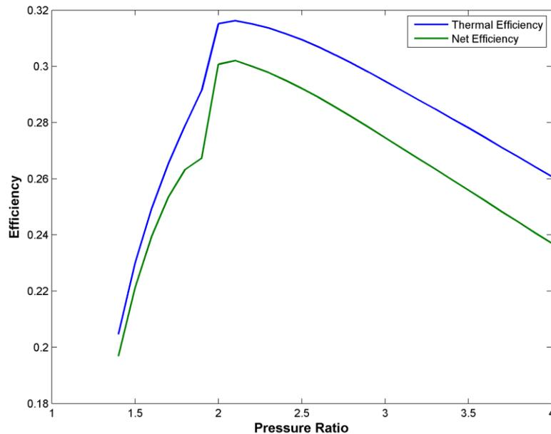
Figure 4 The pressure ratio effect on cycle efficiency
