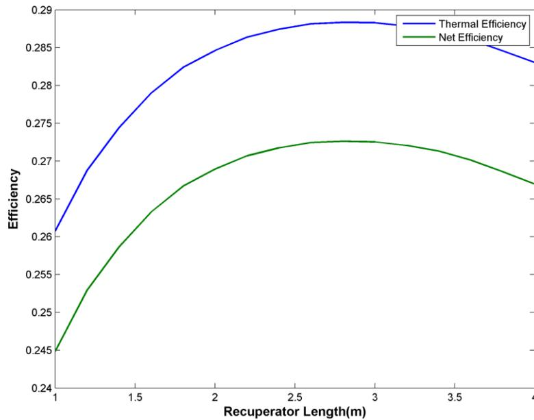
Figure 7 The recuperator length effect on cycle efficiency
