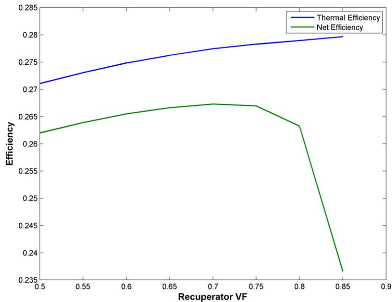
Figure 6 The recuperator volume fraction (VF) effect on cycle efficiency
