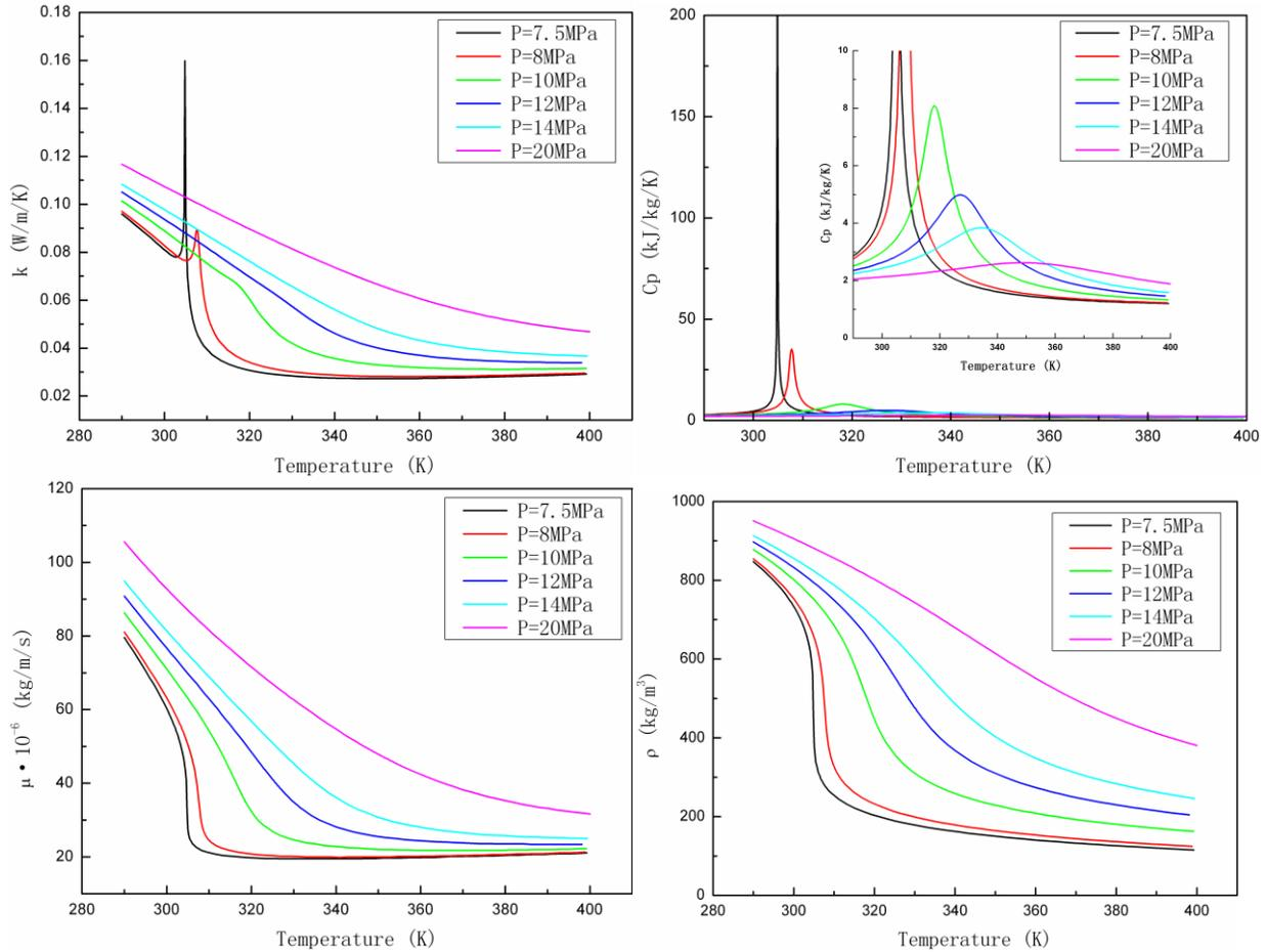
Figure 1 typical fluid properties profile for carbon dioxide
