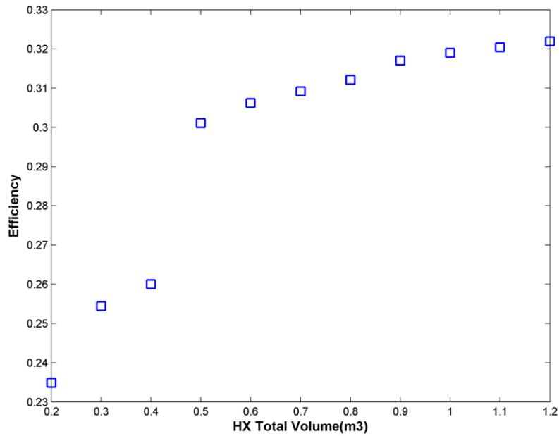
Figure 9 The heat exchanger(HX) total volume effect on cycle efficiency
