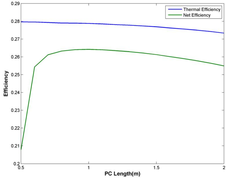
Figure 8 The pre-cooler length effect on cycle efficiency
