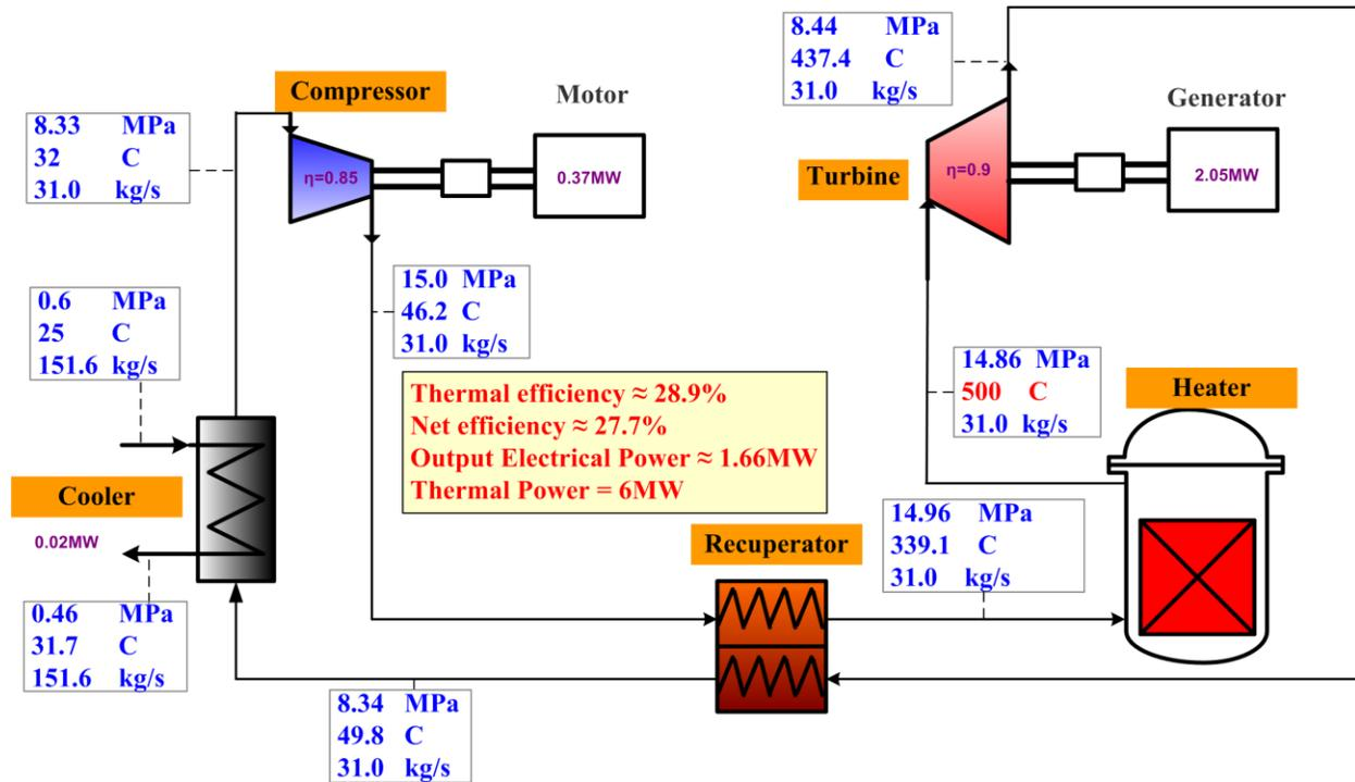
Figure 10 The thermal diagram for MW class loop (conceptual)
