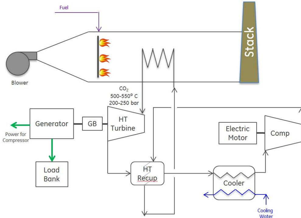
Figure 4 Simple Recuperated Cycle
