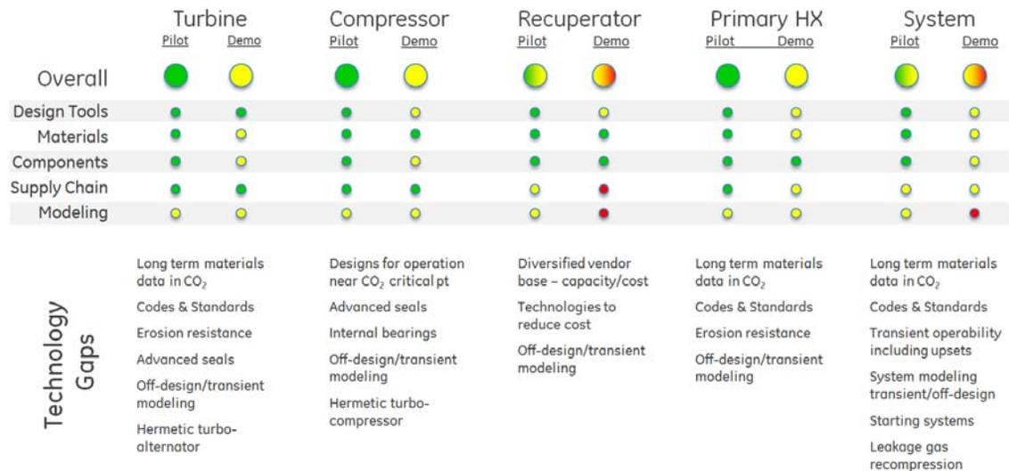
Figure 2 Technology gaps for 550C CO<sub>2</sub> power cycles
