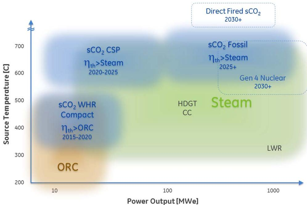
Figure 1 Application space for CO<sub>2</sub> power cycles
