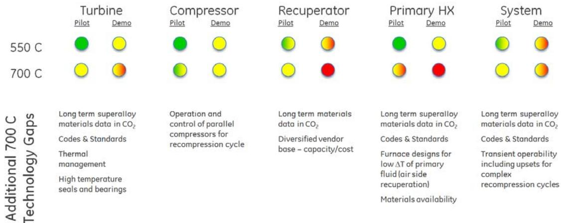
Figure 3 Technology gaps for 700C CO2 power cycles
