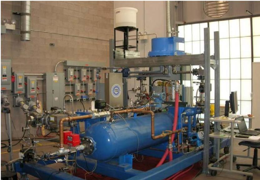
**sCO<sub>2</sub> Bearings, Seals and Compressor research platform**
