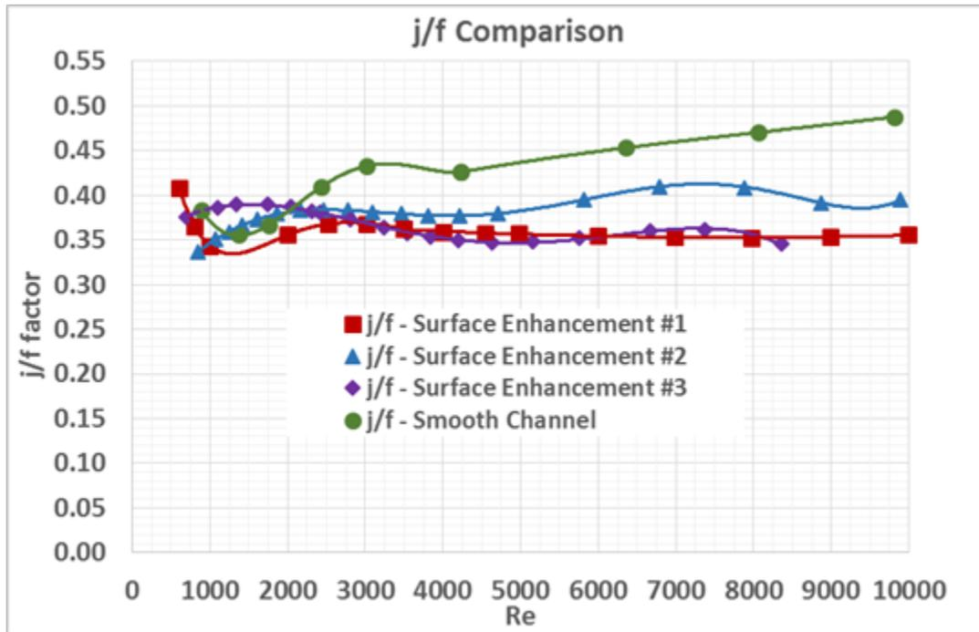
Figure 6 – Comparison of  $J/f$  for Smooth Channel and Surface Features 1, 2 and 3 Cases
