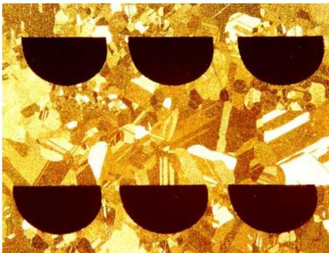
**Figure 2 – Diffusion Bonded PCHE Cross-Section Picture**
