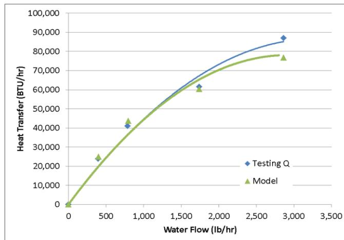
**Figure 7 – Comparison of Early Inserts HELC Heat Transfer Test Data and Model Results**
