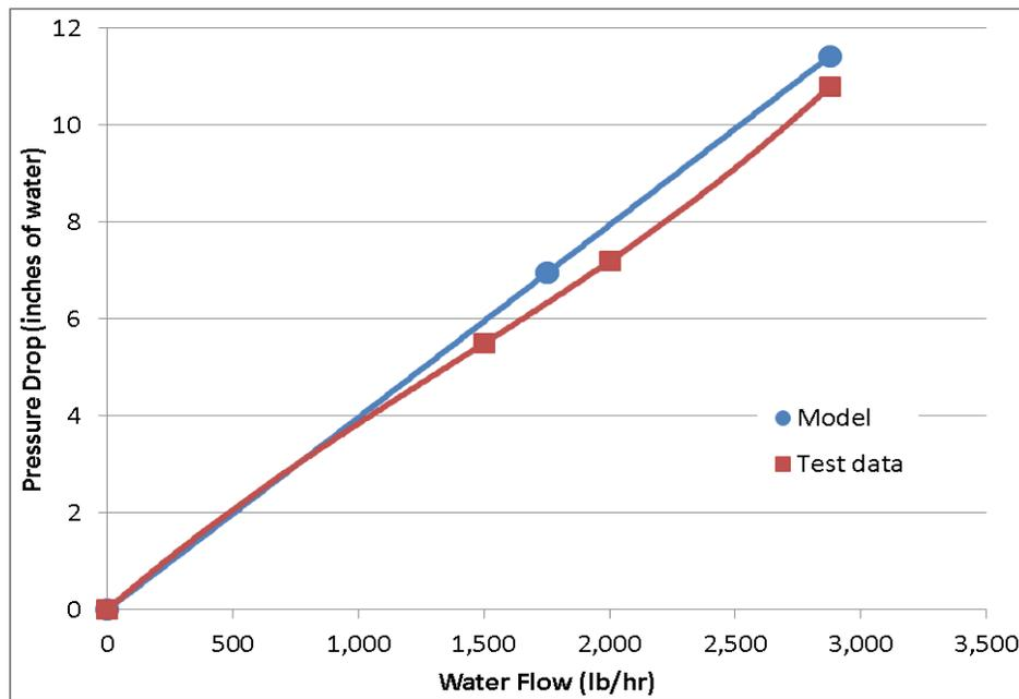
**Figure 8 – Comparison of Early Inserts HELC Test and Model Pressure Drop Results**
