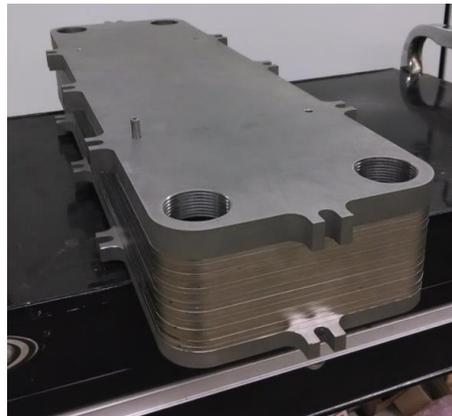
**Figure 4 – HELC 30 KWt Test Article with Early Inserts**
