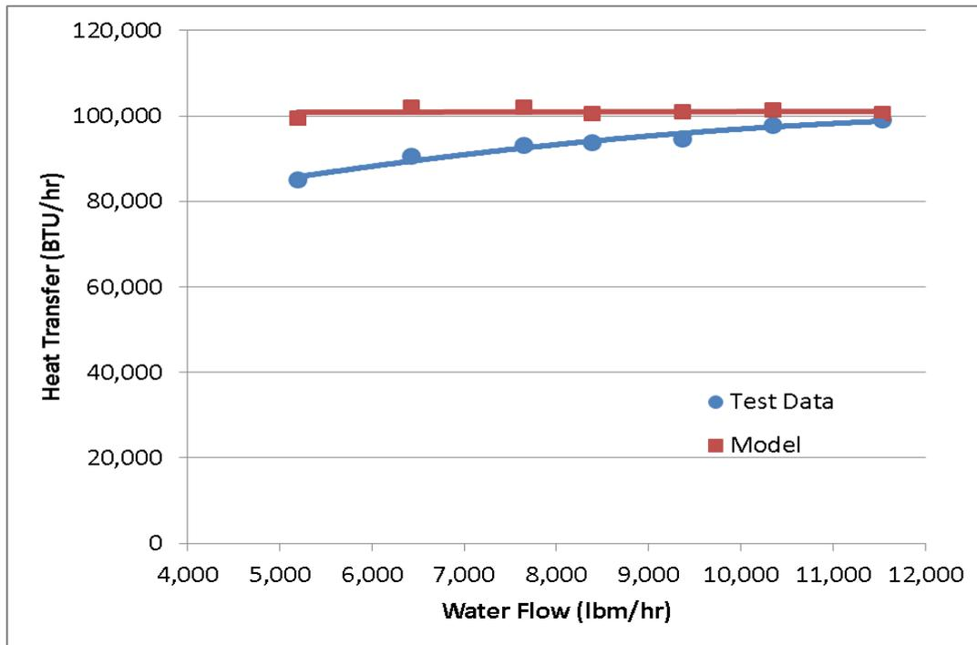
**Figure 10 – Comparison of Updated 30 KWt HELC Article Test and Model Heat Transfer Results**
