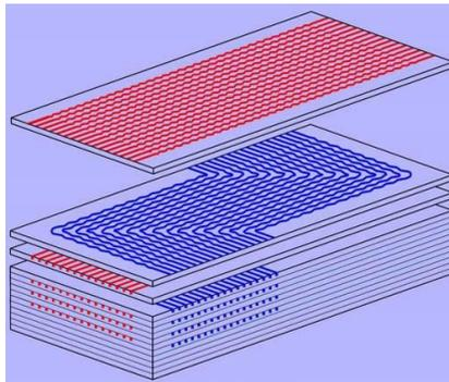
**Figure 1 – Chemically Etched Channels in Stacked Plates**
