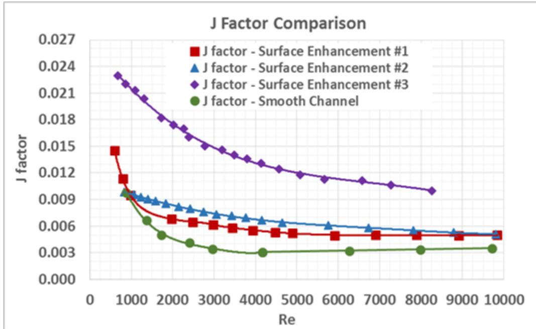
Figure 5 – Comparison of Smooth and Surface Feature Enhancements 1, 2 and 3 for HELC
