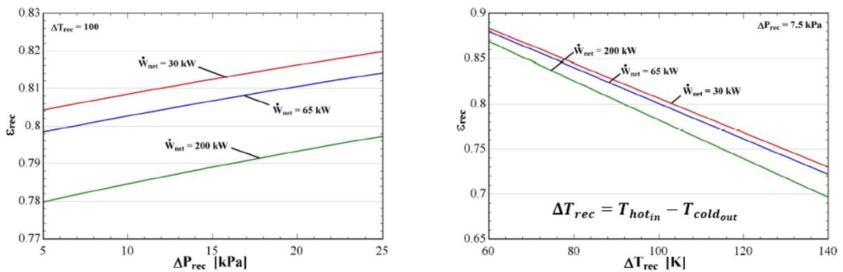
Figure 5 Heat exchanger plate effectiveness as a function of pressure drop (left) or approach temperature (right).
