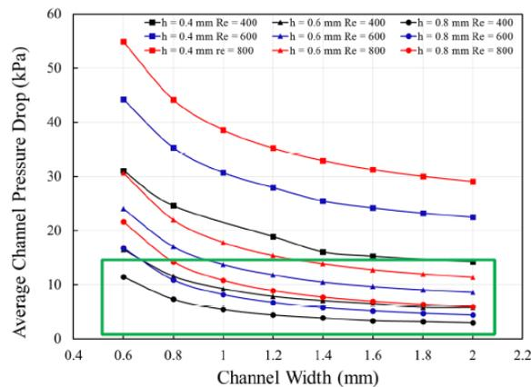
Figure 4 Channel pressure drop versus width for several Reynolds numbers and channel heights.
