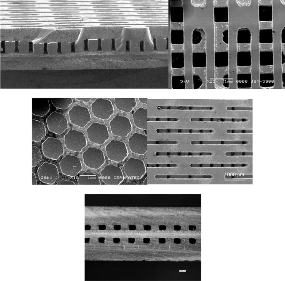
Figure 3 Examples of microchannel features produced by laser featuring. formed by laminating the featured or unfeatured layers together using combinations of heat and pressure. Plates are subject to a thermal cycle that removes the organic binders and plasticisers and then densifies the components via sintering, resulting in components that can be joined together to form the modular stacks described earlier, see Figure 3. As an example of the compact size of these
