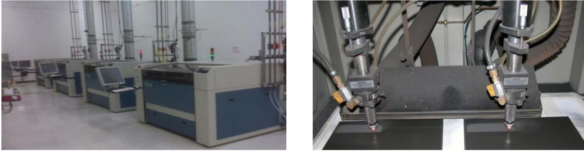
Figure 2 Typical laser featuring equipment (a), and (b) their operation, used to produce microchannel layers.
