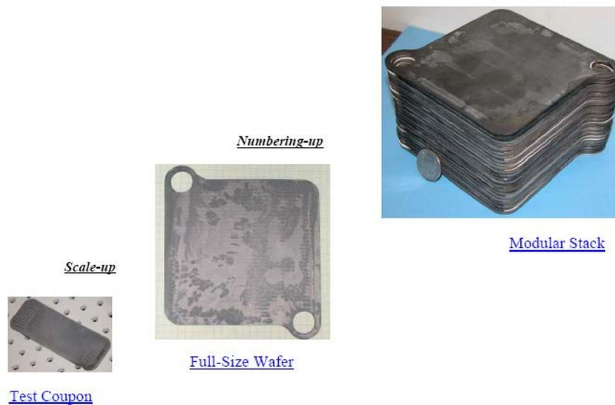
Figure 1 Modular stack design of a ceramic, compact heat exchanger.
