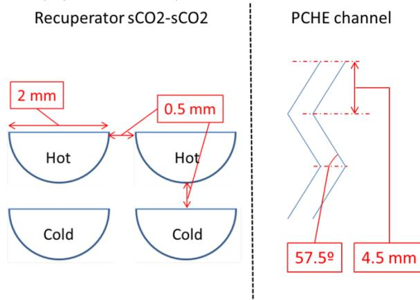
**Figure 5: Basic geometry of reference PCHE.**
