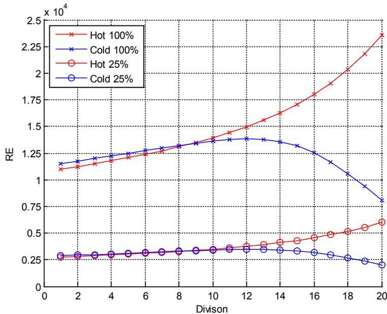
**Figure 8: Average Reynolds number on both sides as predicted by the PCHE model at various load settings. In this figure, the hot side of the heat exchanger flows from left to right while the cold side of the heat exchanger flows right to left.**
