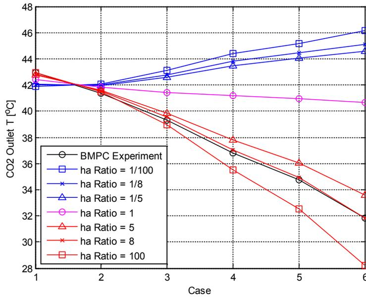
**Figure 1: CO2 outlet temperature for several off-design cases of the sCO2/water heat exchanger from BMPC along with predicted performance using our method for various values for  $hA_{ratio}$ .**
