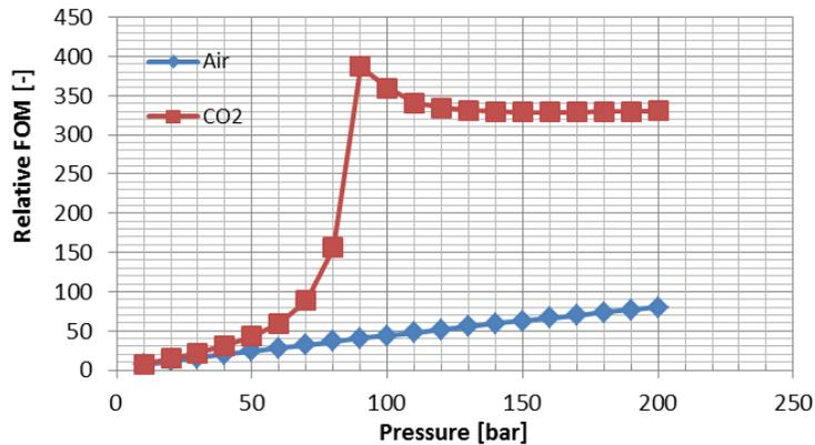
Figure 6: The comparison of relative figure of merit (convection) between air and CO<sub>2</sub> as a function of pressure.
