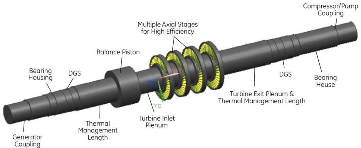
**Figure 9: Final SunShot sCO<sub>2</sub> turbine rotor design**
