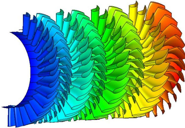
**Figure 4: Airfoil designs for 4-stage SunShot turbine**
