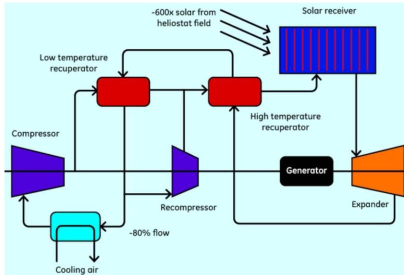
**Figure 1: Recompression sCO<sub>2</sub> Cycle**
