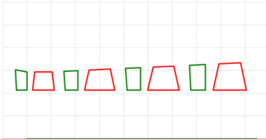
**Figure 3: Preliminary flow path layout of the 4-stage axial turbine**
