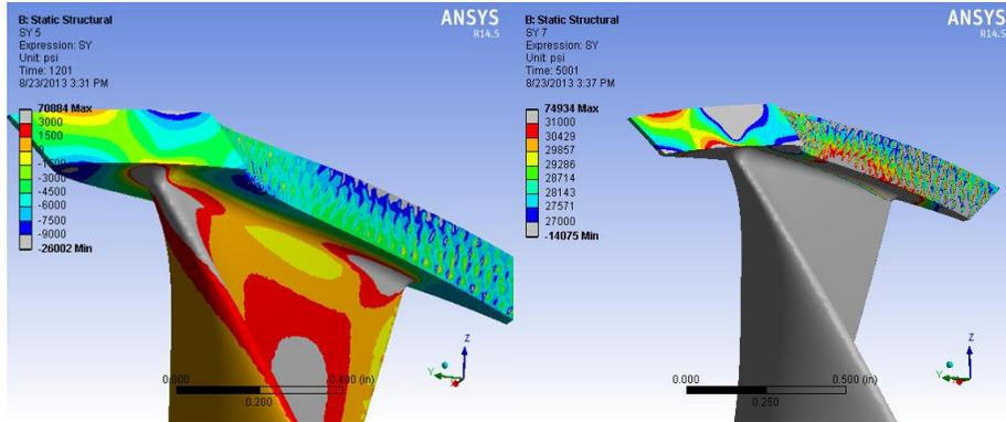
**Figure 8: Peak equivalent stress profile in the turbine blade and shroud for (a) After transient to full rated conditions (centrifugal + thermal) and (b) After cool down due to cloud transient (centrifugal + thermal)**
