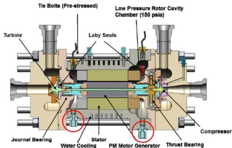
**Figure 6: A cross-sectional diagram of the turbo-alternator-compressor (TAC) unit. Two drain locations are shown on the bottom of the unit (circled in red), with one drain line currently unused and closed off by the Swagelok fitting shown in Figure 7**
