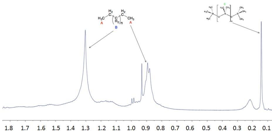
**Figure 8: NMR spectrum of tar dissolved in hexane. The first two peaks correspond to a hydrocarbon oil such as Welch DuoSeal Pump Oil as shown in the spectrum of the oil alone in Figure 9. The third peak corresponds to silicone oil such as Fisherbrand Silicone Oil shown alone in the spectrum in Figure 10.**
