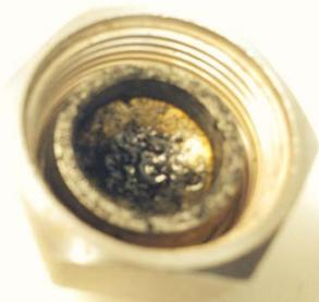
**Figure 7: Swagelok cap with fouling product from the turbo-alternator-compressor (TAC) unit in the RCBC.**
