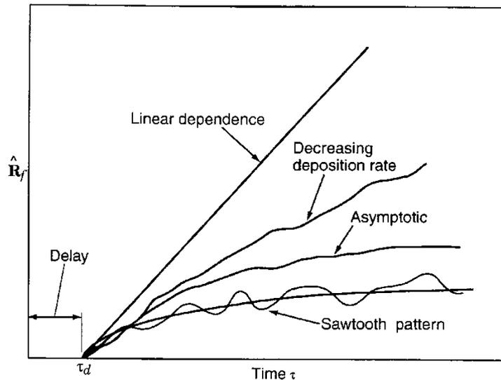
**Figure 2: Typical fouling behavior trends for heat exchangers [1].**
