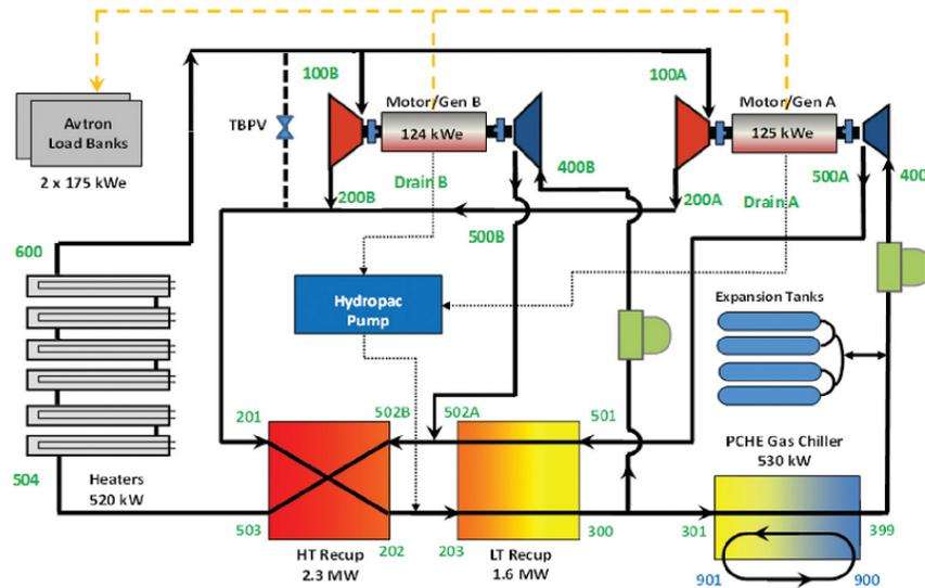
Figure 1: Schematic diagram of the SCO<sub>2</sub> RCBC test article.
