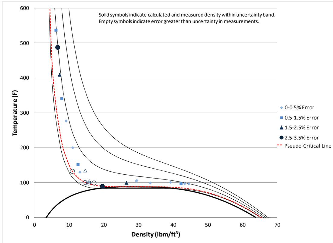
**Figure 4. Difference in Measured and Calculated Density During IST Operation**
