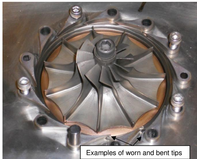
**Figure 3. Turbine Nozzle Wear**
