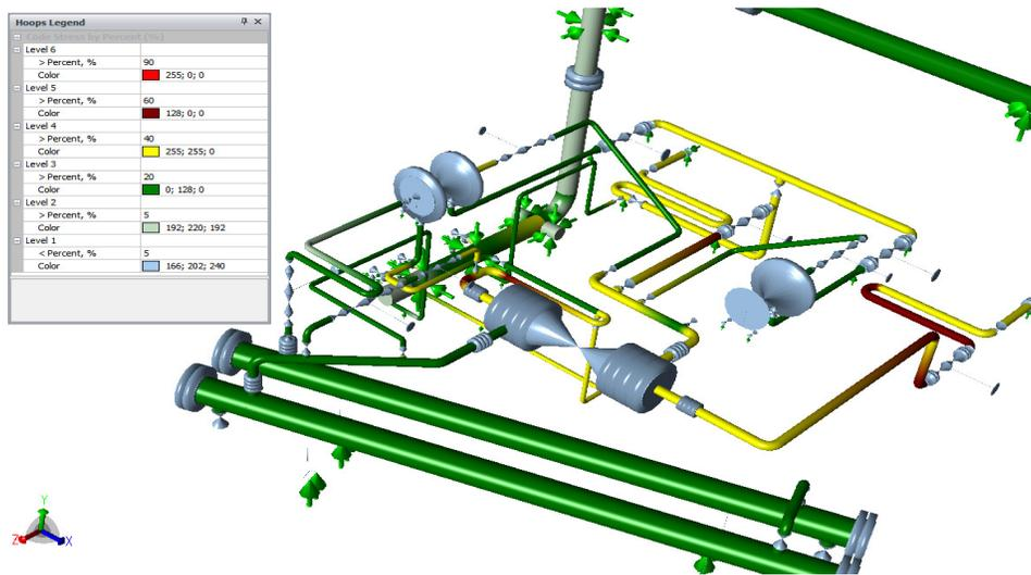
**Figure 2. Thermal Stress Analysis of Brayton Loop Piping**
