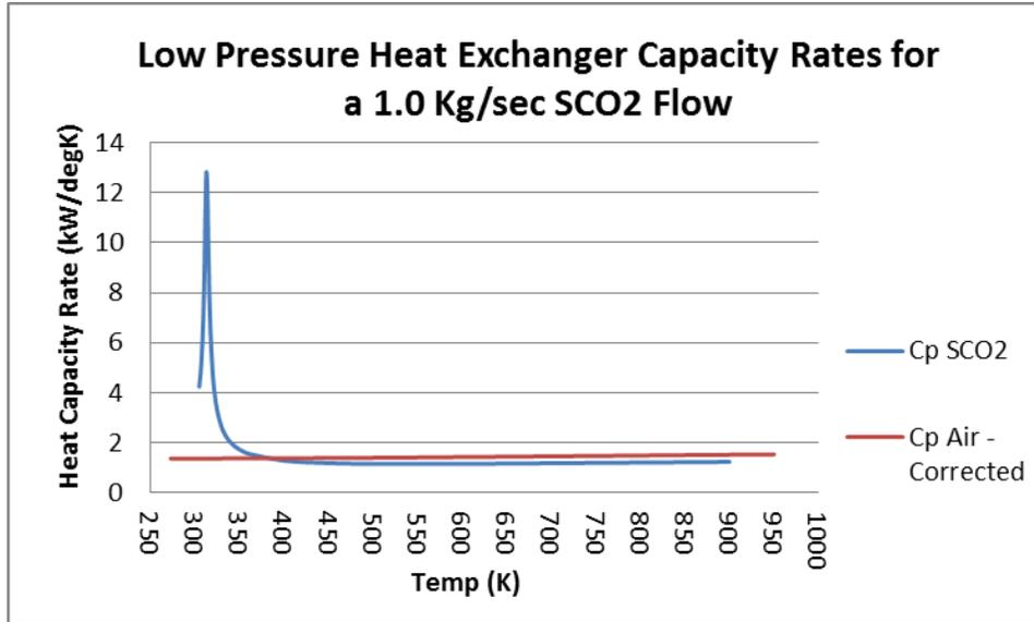
Fig. 3 Heat Capacity Rates for Low Pressure HX
