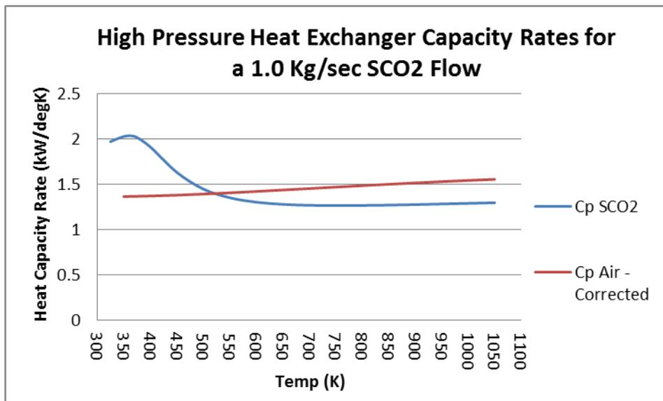
**Fig. 4 Heat Capacity Rates for High Pressure HX**
