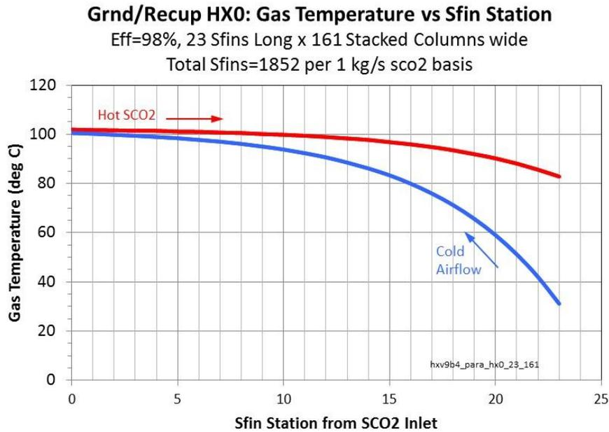
**Fig. 7 Large Delta Temperature Alleviates Pinch Point**
