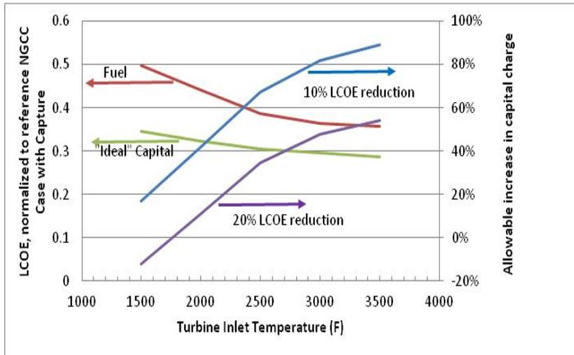
Figure 9: Allowable Capital Cost Increase to Reach Target LCOE Reductions for Directly Fired Cycle
