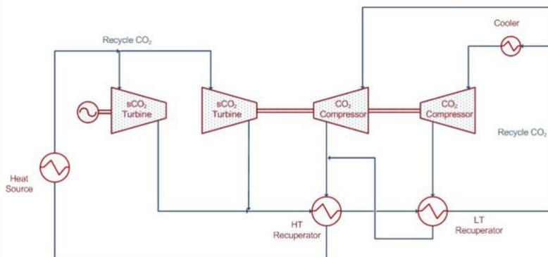
Figure 1: Indirectly Heated Recompression Brayton Cycle
