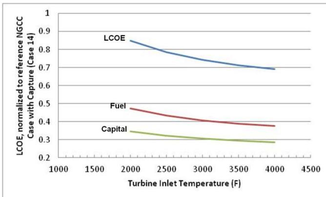
Figure 7: Idealized Decrease in LCOE as a Function of TIT - Directly Heated Cycle
