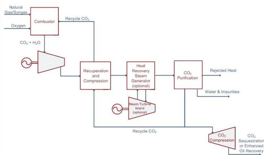
Figure 2: Directly Heated Recuperated Brayton cycle
