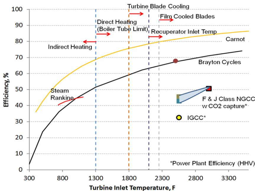
Figure 3: Gross Efficiency as a Function of Turbine Inlet Temperature
