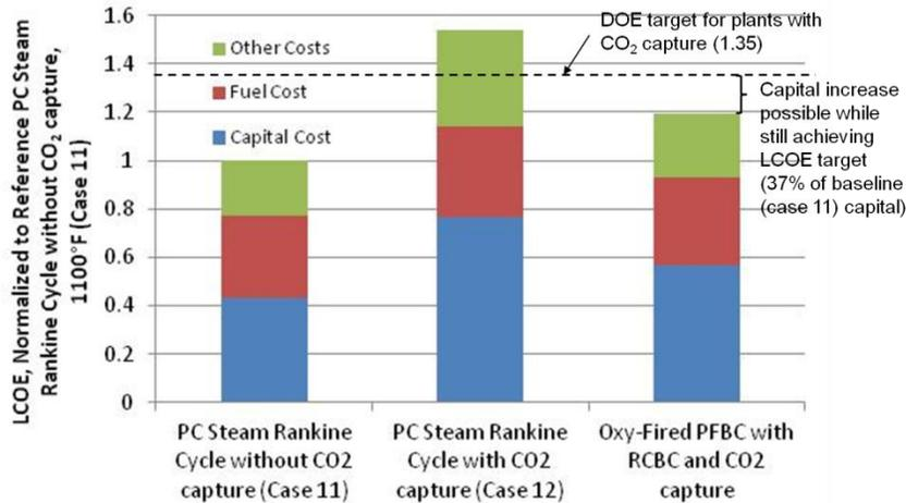
Figure 6: LCOE for Indirectly Fired Cycles
