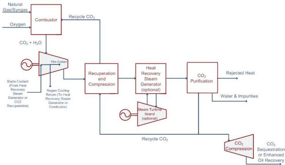
**Figure 4: Directly Heated Cycle with Turbine Blade Cooling**
