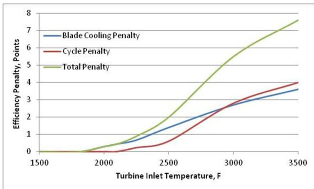
Figure 8: Efficiency Penalties to Mitigate Temperature Constraints
