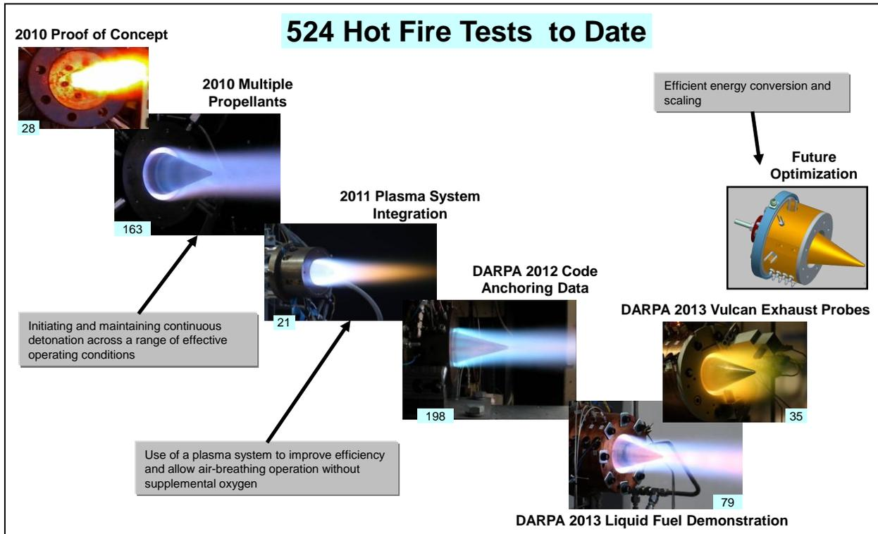
**Figure 3. Aerojet Rocketdyne has Steadily Matured RDE Technology**
