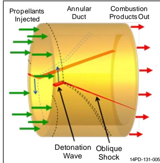
**Figure 2. Schematic of a Rotating Detonation Engine**
