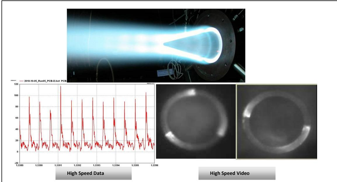
**Figure 4. Aerojet Rocketdyne RDE Test Successes: RDE Operating with Aerospike Nozzle (Top), high frequency pressure signal indicates repeatable detonation waves achieved (bottom left), multiple rotating waves seen in flow visualization (bottom right)**
