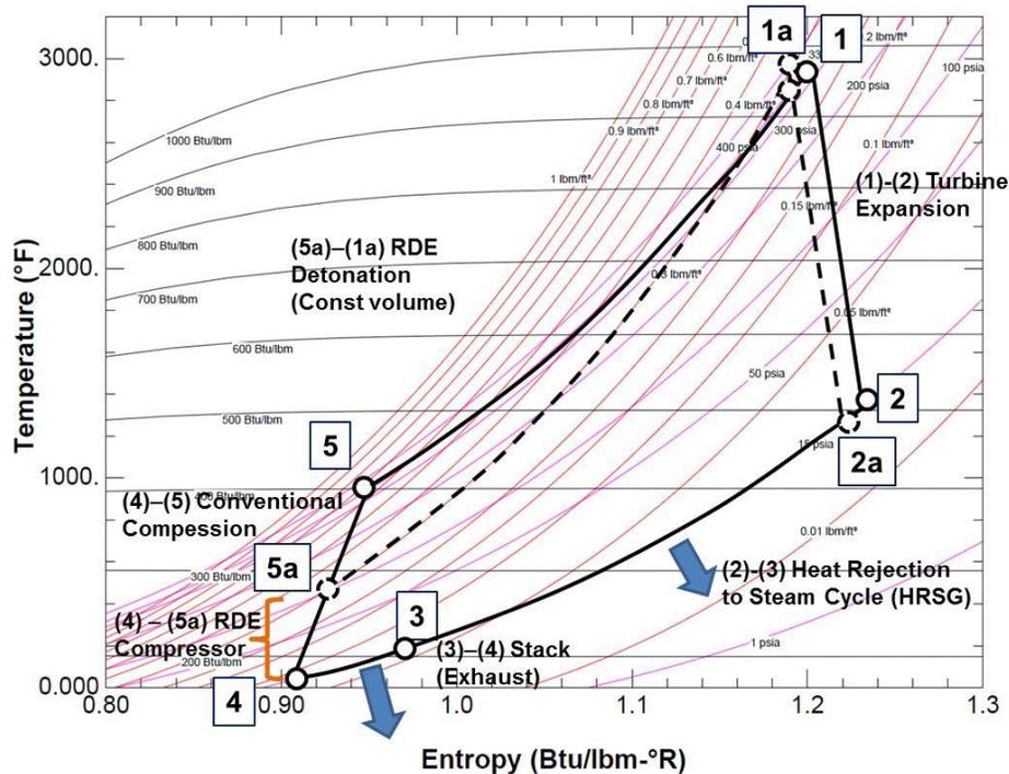
**Figure 1. Mitsubishi Heavy Industries Commercial J Class turbine NGCC has been used as an example to compare conventional constant pressure adiabatic combustion turbine with pressure gain combustion using rotating detonation engine.**
