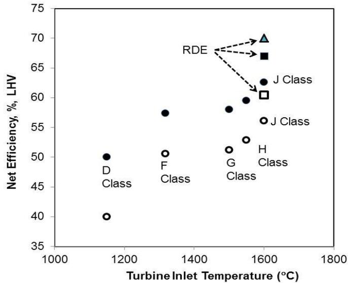
Figure 8. Net plant efficiency of various commercial combined cycle power plants without (filled circles) and with CO<sub>2</sub> capture (open circles) (Wally Shelton, DOE/NETL-341/061013). The RDE based J class NGCC plant with and without capture is shown with open-square and filled squares. The RDE based RCBC sCO<sub>2</sub> cycle is shown as filled triangle.
