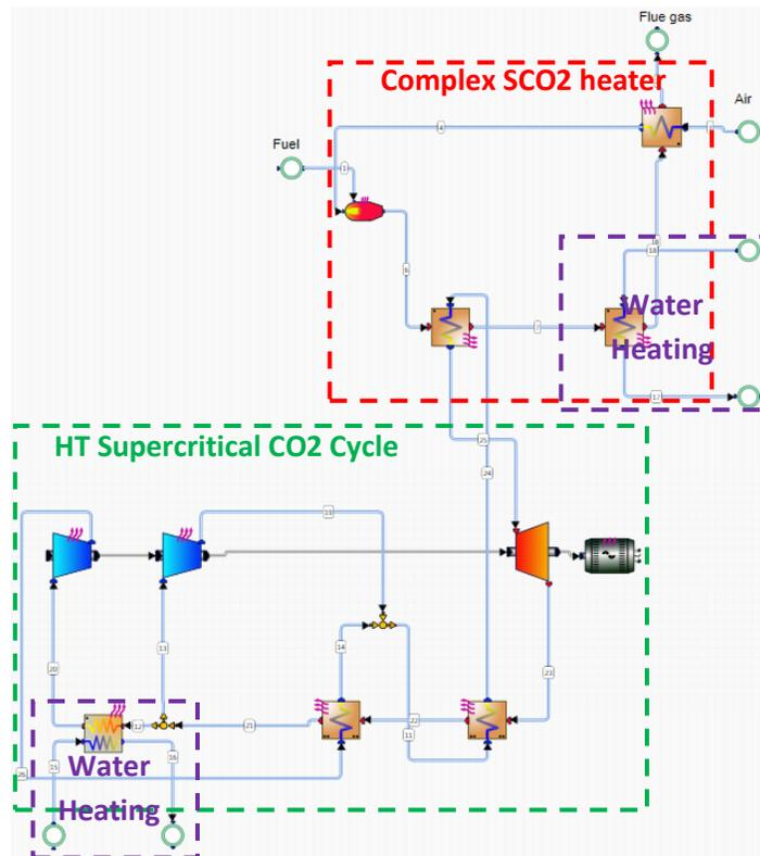
Figure 6. Single Supercritical CO<sub>2</sub> CHP Plant
