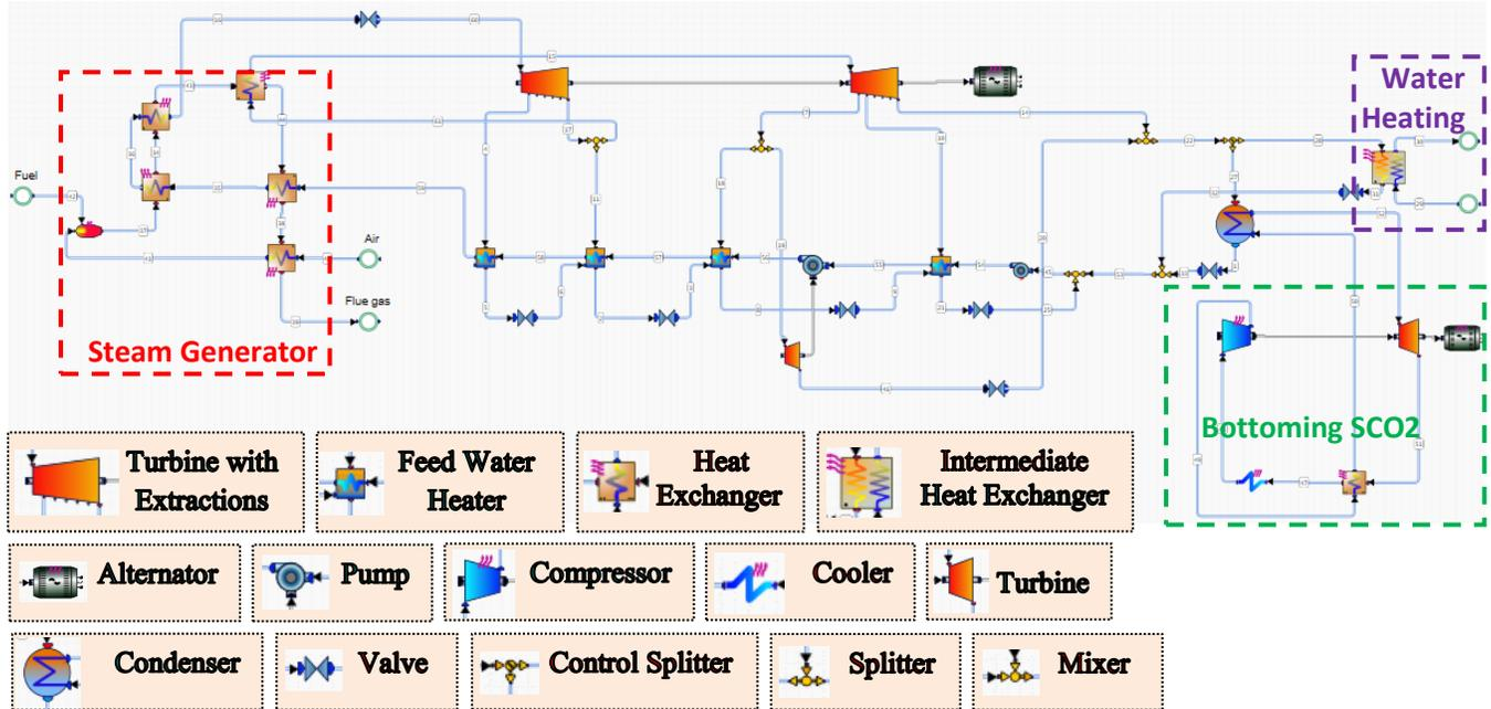
Figure 3. Combined Complex Steam-SCO<sub>2</sub> CHP Plant
