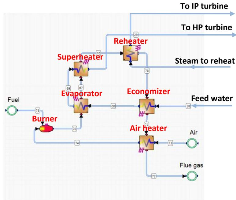
Figure 2. Fossil Fuel Fired Water Steam Generator.
