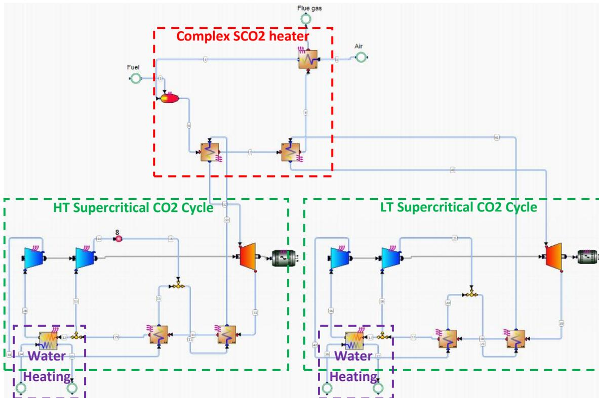
Figure 5. Cascaded Supercritical CO2 CHP Plant
