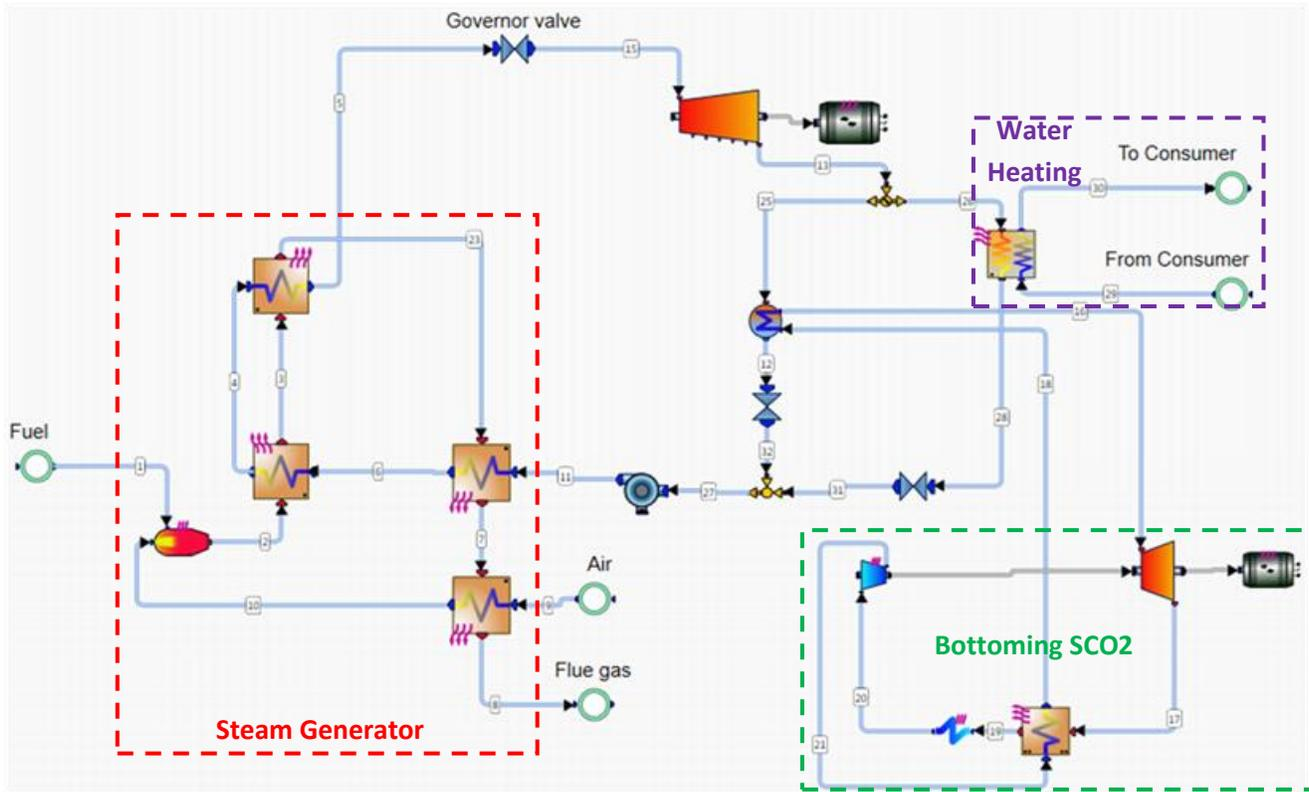
Figure 4. Combined Simple Steam-SCO<sub>2</sub> CHP Plant
