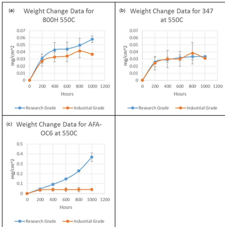
Figure 2: Weight gain data for tests performed in SC-CO<sub>2</sub> at 550°C and 2900psi, (a) 347 stainless steel (b) alloy 800H and (c) AFA-OC6.
