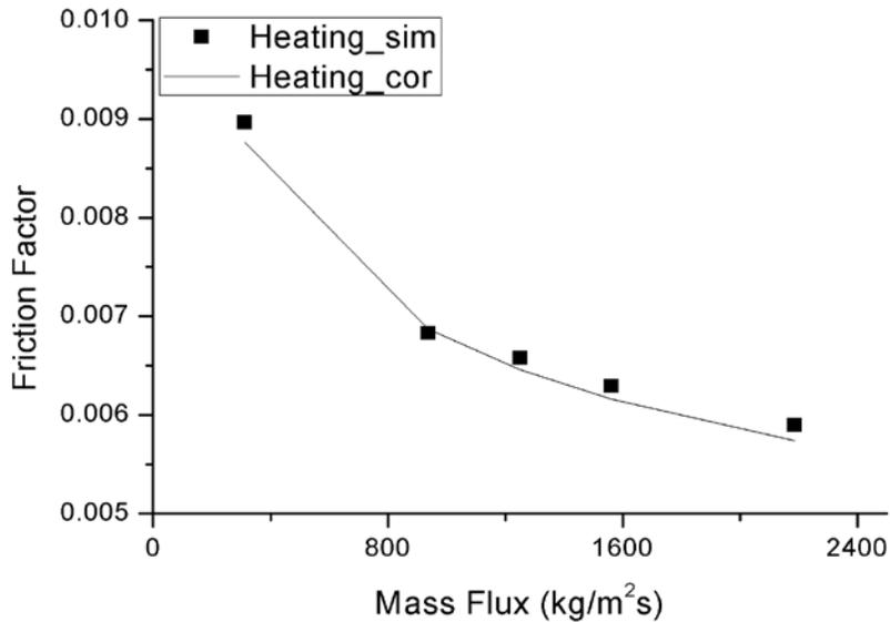
Figure 6. Friction factor variation with variation of mass flux
