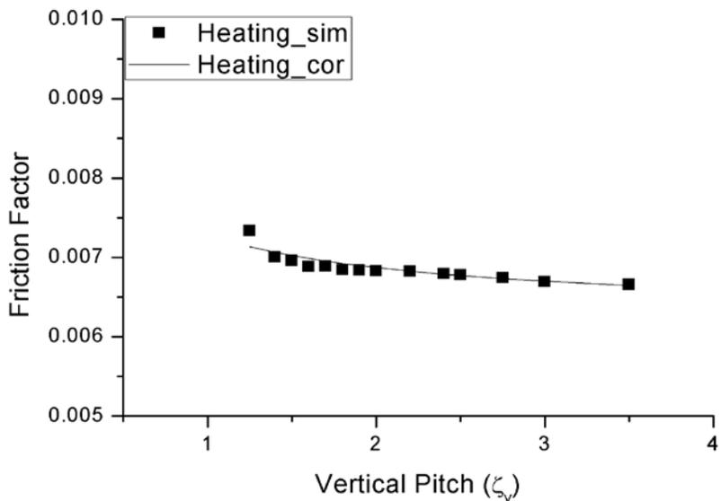
Figure 7. Friction factor variation with variation of vertical pitch
