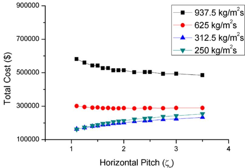
Figure 11. Total cost of the recuperator with horizontal pitch variation
