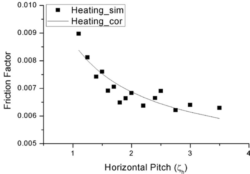
**Figure 8. Friction factor variation with variation of horizontal pitch**
