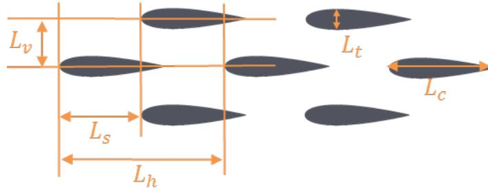
Figure 2. Geometrical parameters of airfoil array
