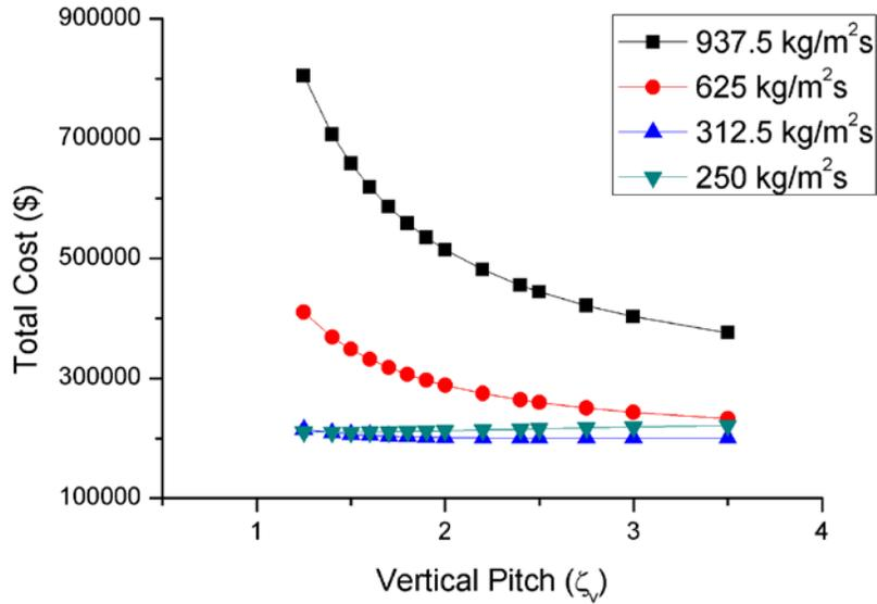
Figure 10. Total cost of the recuperator with vertical pitch variation
