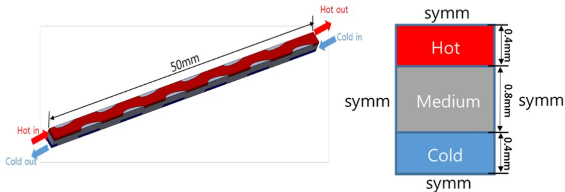
**Figure 1. Schematic of simulation domain and boundary conditions**
