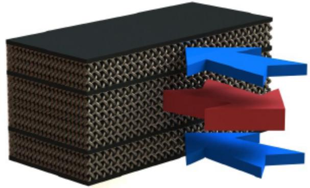
Figure 2 Rendering of a detail of the wire-mesh heat transfer surface and the associated flows
