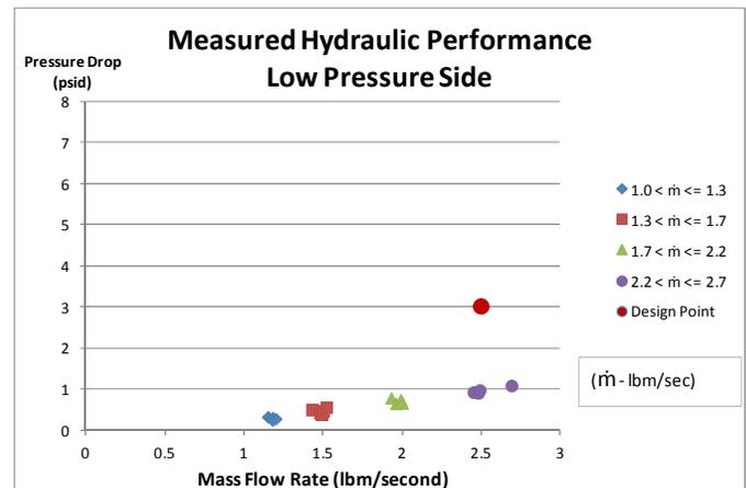
Figure 9 Measured hydraulic performance for the low pressure side of the recuperator using the traditional, folded-wavy-fin heat transfer surface
