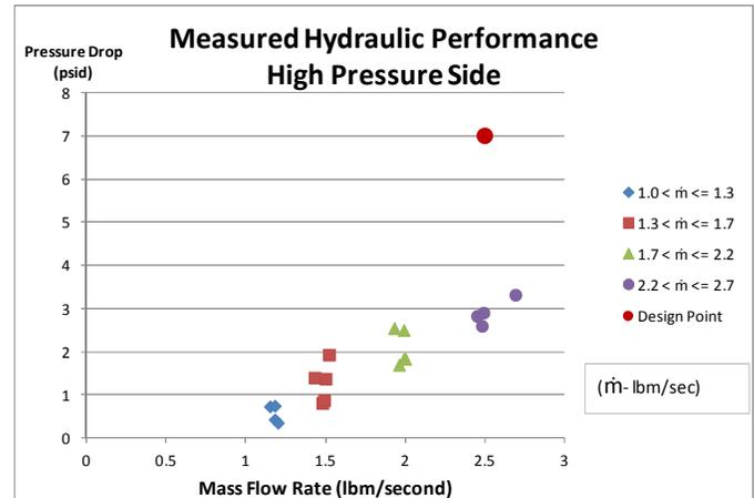
Figure 8 Measured hydraulic performance for the high pressure side of the recuperator using the traditional, folded-wavy-fin heat transfer surface
