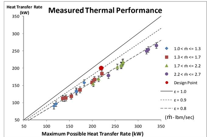
Figure 7 Measured thermal performance showing the effectiveness of the recuperator using the traditional, folded-wavy-fin heat transfer surface
