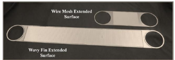
Figure 3 Photograph of wire-mesh unit-cell side-by-side with a folded-wavy-fin unit-cell
