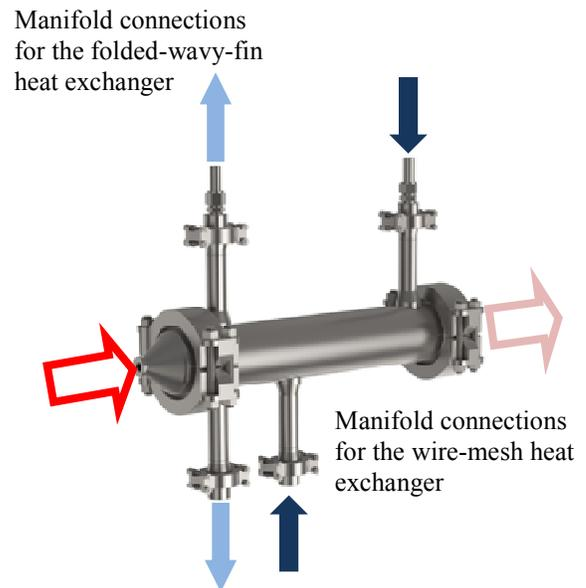
Figure 5 Rendering of the test section for the small-scale heat exchangers (see legend in Figure 3)
