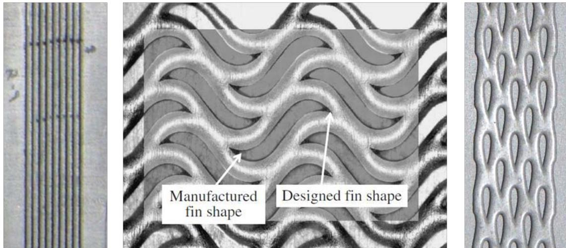
**Figure 5. Traditional (far-left), s-shaped fin, and airfoil fin PCHE surface geometries. Directly casting a heat exchanger with flow channels similar to the s-shaped and airfoil fin surfaces could be done using casting cores reminiscent of perforated plates.**
