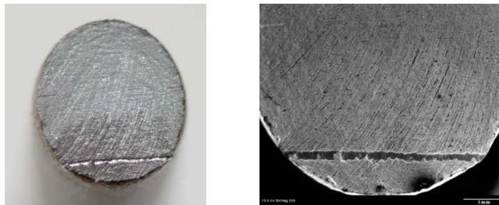
**Figure 4. Photograph and SEM image of one side of the failure surface of sample A. The trench shown is likely the result of a foreign object inclusion leading to premature failure.**
