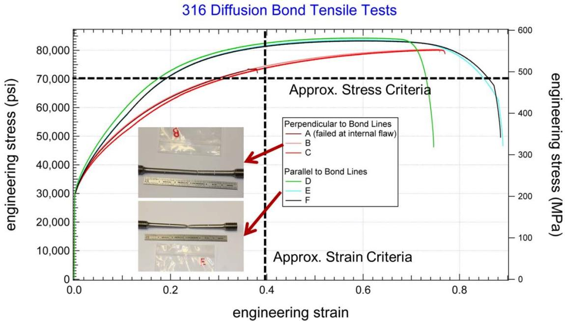
**Figure 3. Stress-strain curves from the first set of 316L diffusion bond samples. Minimum stress and strain criteria are overlaid on the plot, with all but sample A meeting criteria.**
