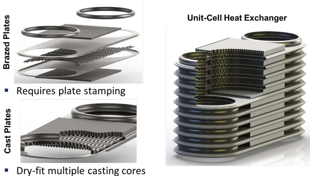
Figure 7. A comparison of the plate processing steps involved in producing a unit-cell heat exchanger using either bonded brazed or directly-cast plates. For the cast plates, finned or island-style surfaces would need to be used rather than the discrete sinusoidal channels shown.
