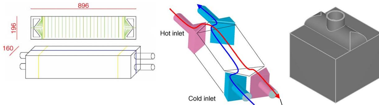
**Figure 2. Configuration of the Heatric PCHE tested by Pra et al. (Pra et al., 2008) with V-style headers on the left, as compared with the petal-style header (ALPEMA, 2010).**
