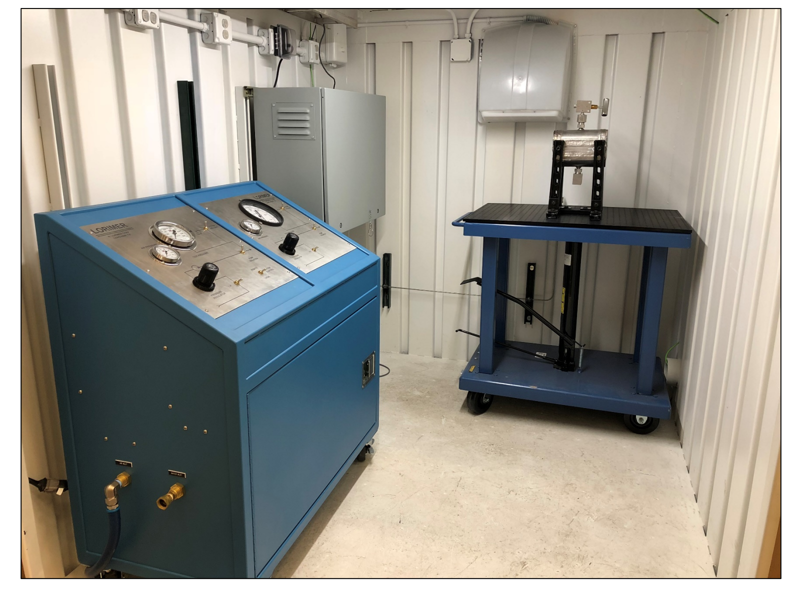
Pressure Vessel Failure Modes Experiment with hydrostatic pressure cart, data acquisition and control in electrical enclosure, and header prototype inside secondary containment shipping container
