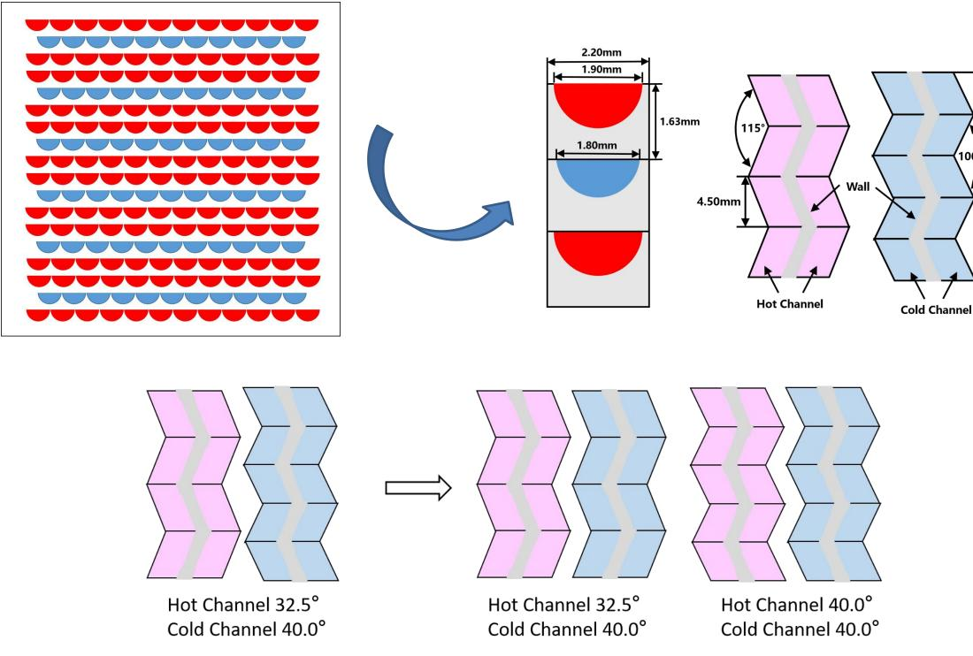
The top and bottom, left and right surfaces of PCHE are set as translational periodicity boundary condition and the front and rear surfaces are set as adiabatic boundary conditions. For the boundary layer between PCHE and SCO2 fluid, general connection was used. The first-order high-precision convergence mode was adopted and the convergence precision is 10-4.
