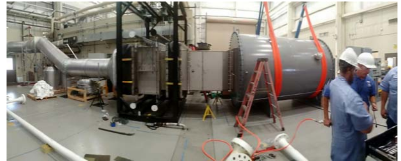
Heat Exchanger with the Associated Support Structure, Spring Can Supports, Expansion Joints, etc.
