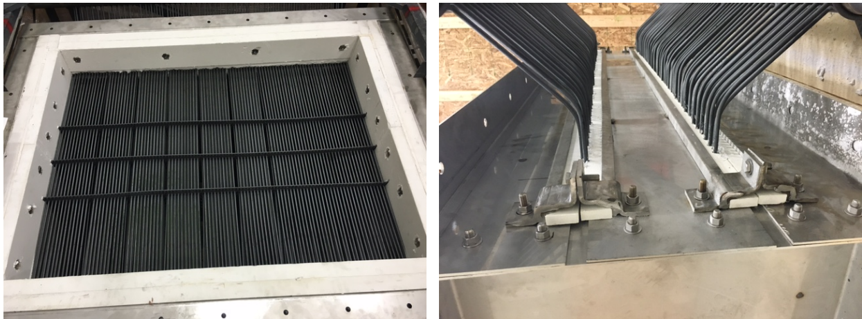
Figure 10. Heater Heat Exchanger
