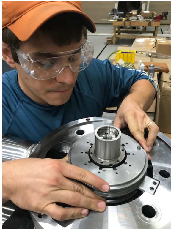
Figure 5. Turbine Assembly Showing Thrust Bearing Installation
