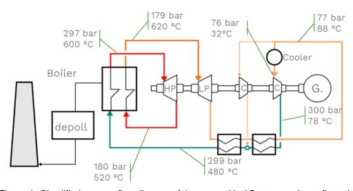
Figure 4: Simplified process flow diagram of the supercritical Brayton cycle configuration
