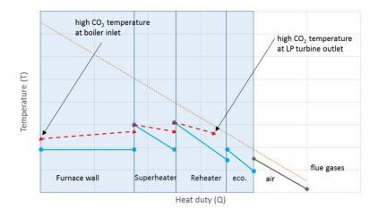
Figure 2: Coal-fired power plant qualitative T-Q diagram (dotted orange = flue gas, blue = water, dashed red =  $CO_2$  and gray = air)
