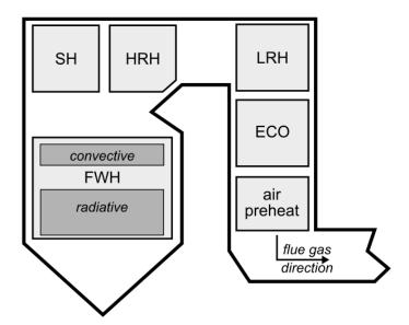
Figure 3: simplified diagram of considered coal-fired heater
