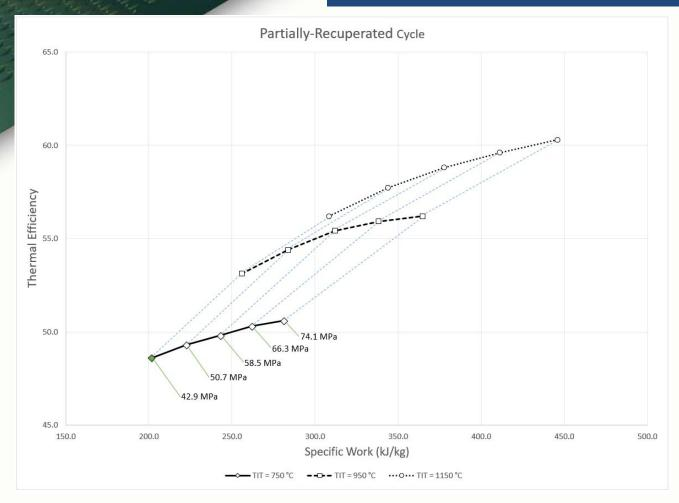
Temperature Capability of Primary Heat Exchangers is Limiting Rather Than That of the Turbine Wheel
