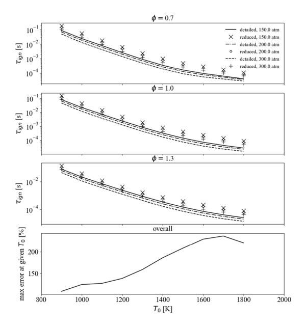
Figure 2. Comparison of autoignition delays at different conditions between the detailed kinetic model and the reduced kinetic model before optimization and their associated errors
