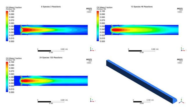
Figure 12 O<sub>2</sub> mass fraction contours of the global 5 species kinetic model from Fluent, the optimized 13 species kinetic model from USC Mech II, and the 24 species kinetic model from GRI Mech 3.0
