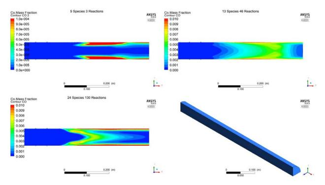
Figure 13 CO mass fraction contours of the global 5 species kinetic model from Fluent, the optimized 13 species kinetic model from USC Mech II, and the 24 species kinetic model from GRI Mech 3.0 (different scale for 5 species model)
