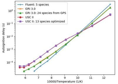
Figure 4. Autoignition delay of different temperatures for different kinetic models with 200 bar and stoichiometric equivalence ratio (94.13% CO<sub>2</sub> dilute)
