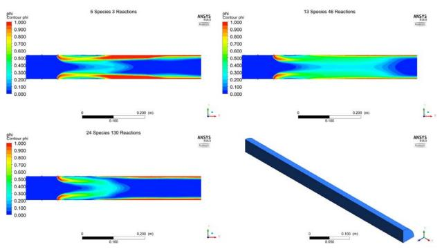
Figure 15 Normalized equivalence ratio contours of the global 5 species kinetic model from Fluent, the optimized 13 species kinetic model from USC Mech II, and the 24 species kinetic model from GRI Mech 3.0 model
