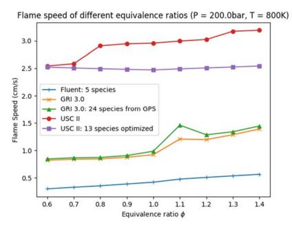
Figure 5 Laminar flame speed (unit: cm/s) of different equivalence ratios for different kinetic models with 200 bar and initial temperature 800K
