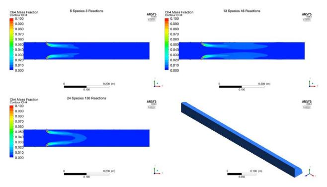
Figure 11 CH<sub>4</sub> mass fraction contours of the global 5 species kinetic model from Fluent, the optimized 13 species kinetic model from USC Mech II, and the 24 species kinetic model from GRI Mech 3.0
