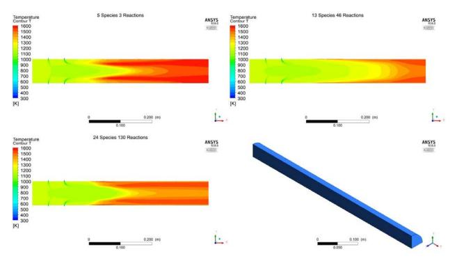
Figure 9 Temperature contours of the global 5 species kinetic model from Fluent, the optimized 13 species kinetic model from USC Mech II, and the 24 species kinetic model from GRI Mech 3.0
