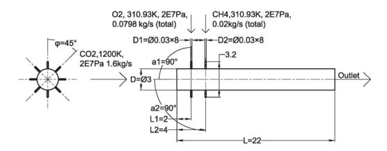
Figure 8. The geometry of crossflow combustor model (unit: inch)
