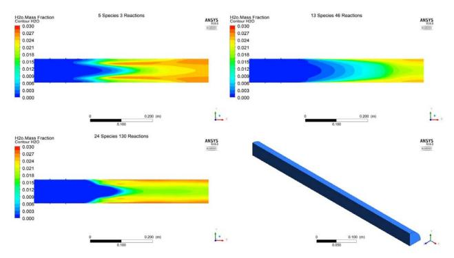
Figure 14 H<sub>2</sub>O mass fraction contours of the global 5 species kinetic model from Fluent, the optimized 13 species kinetic model from USC Mech II, and the 24 species kinetic model from GRI
