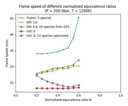
Figure 7 Laminar flame speed (unit: m/s) of different normalized equivalence ratios for different kinetic models with 200 bar and initial temperature 1200K
