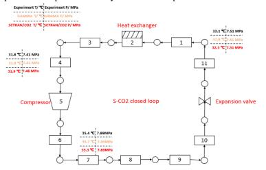
Figure 9 Nodalization of SCTRAN/CO2 model and steady state result at each node
