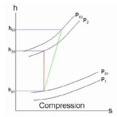
Figure 1 Ideal and realistic compression process inside compressor
