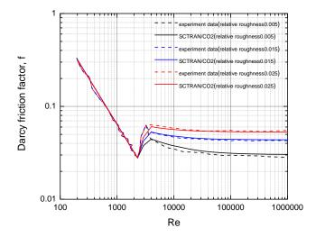
Figure 3 Comparison for friction coefficient of various roughness between experimental data and SCTRAN/CO2 prediction
