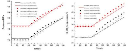
Figure 10 Pressure and temperature variation during the cooling reduction transient
