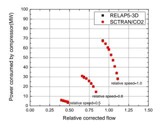
Figure 7 Predicted compressor consuming power by SCTRAN/CO2 and RELAP5-3D
