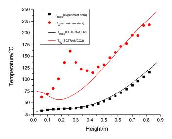
Figure 5 Comparison of bulk temperature and wall temperature of SCTRAN/CO2 result and observed experiment data
