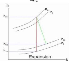
Figure 2 Ideal and realistic expansion process inside gas turbine
