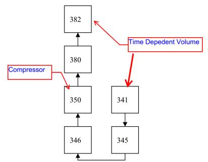
Figure 6 Nodalization of the recompressing compressor
