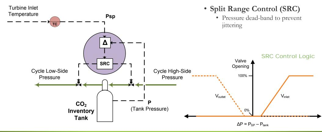
Work Controller (Ratio control augmented w/ feedback trim)
