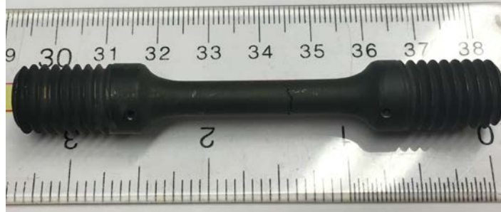
Figure 1: Example specimen profile and associated creep elongation calculation
